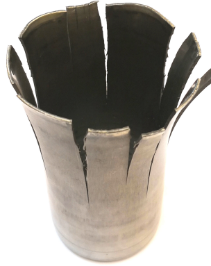
Figure 1.9. Deep drawn cup which has experienced corrosion cracking.
