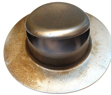
Figure 1.5. Fracture of the cup, due to locally thinning.
