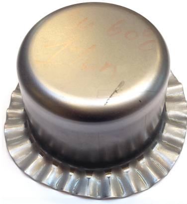
Figure 1.4. Wrinkles appearing on the flange of a deep drawn cup, due to too low blank-holder pressure.
