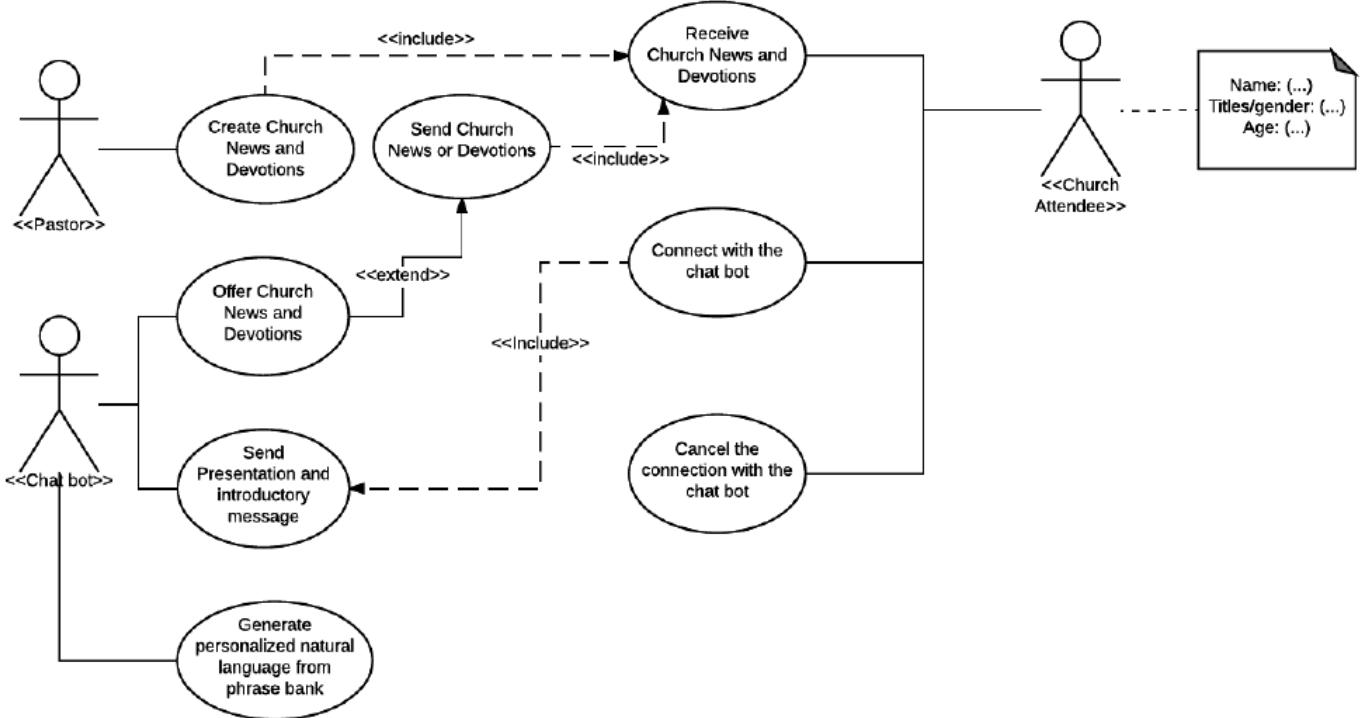
Figure 31: Use Case Diagram of necessary functions in the chat bot and basic entities of a related informal ontology
