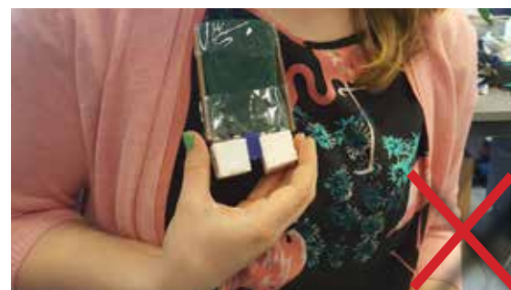
Ill. 62.4 - Activation 2 where the gel lands in the same hand that is used for the squeeze. The hand needs to be in a more angled position, before the gel lands correctly in the palm.
