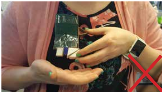
Ill. 62.3 - Activation 1. The container moves to the side when activated. The hand position of the activating hand is a little bit awkward because the hand is pushed towards the chest and the thumb needs to be placed on a edge that sticks out.
