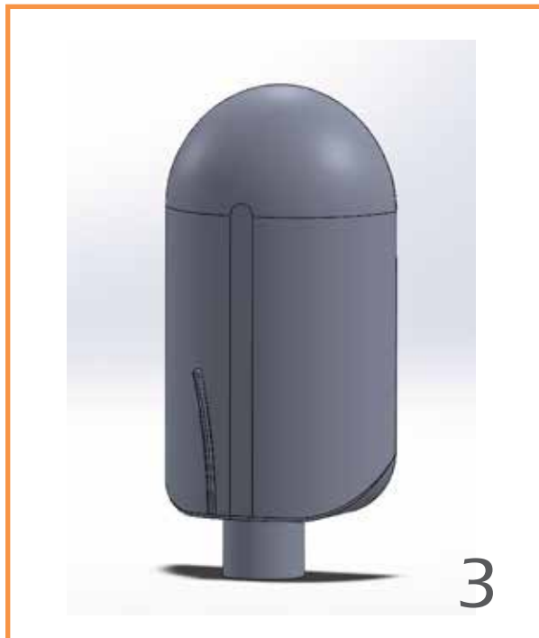
Ill. 77.3 - The third idea is to have rounded edges everywhere except on the back, where it is still flat. The corners are cut off and rounded as well. A guideline that sticks out was added to test if it could be felt.
