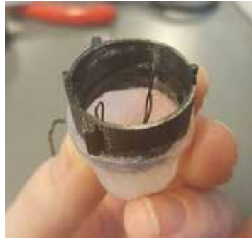
III. 79.2 - The sticks that will cut the foil when the container is turned.
