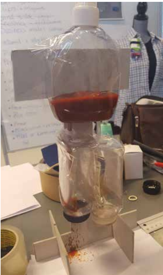
Ill. 85.3 - The setup where the ketchup is pushed out through the valve in the bottom of the left chamber.
