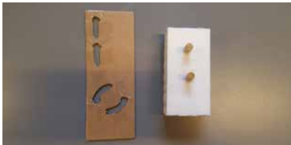
Ill. 52.3 - The mounting was tested with a linear and a rotating mount. The rotating mount created the best illusion of that the container was mounted tightly and would not fall of.
