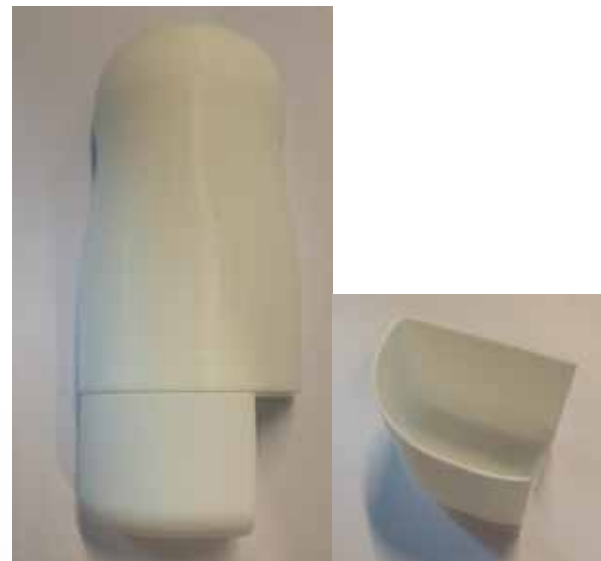
Ill. 81.4 - The 3D printed container and shell attached to each other on the left and the shell viewed from the top on the right.
