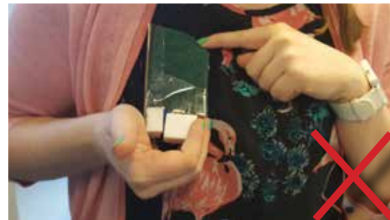
Ill. 62.6 - Based on activation 2, but where the push only happen from one side. A finger needs to be placed on the top of the container so it stays in the right position. There is a slight twist in the elbow when the arm is placed like this.
