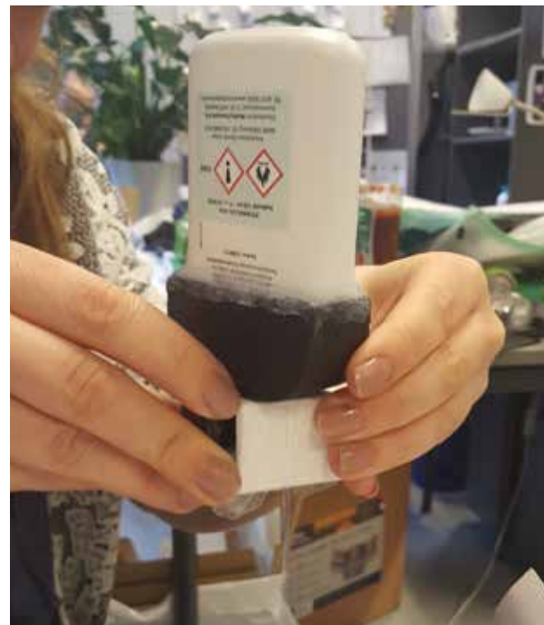
Ill. 73.5 - A mock-up of the solution where the chamber is being squeezed from the side and gel comes out the bottom.
