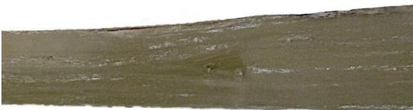
No damage visible. Ply drop remained intact at the other half of the cylinder.
