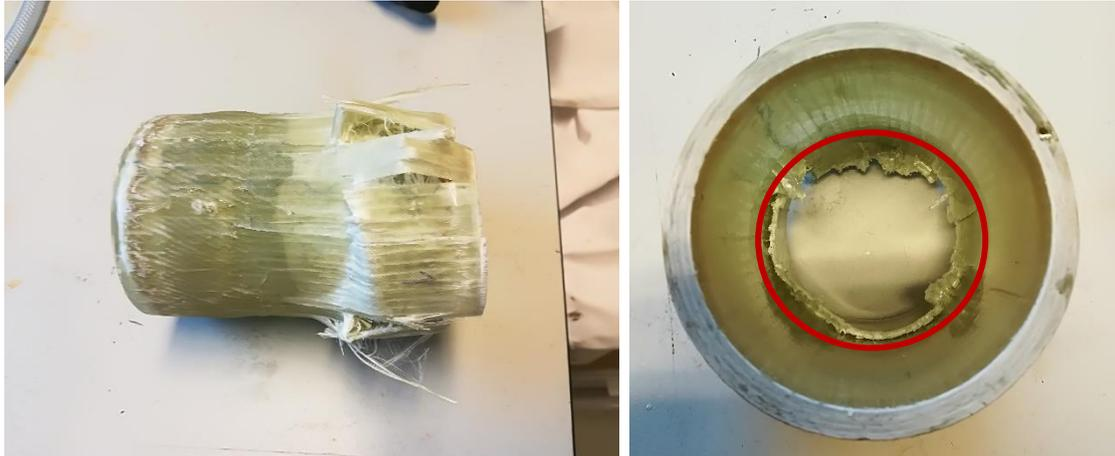
*Figure D.1. Specimen under centered compression after failure. Damage is visible around the whole cylinder.*
