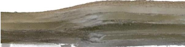
Damage looks similar as at the previous cut. Delamination at the upper layers of the ply drop and fibre failure at the bottom.
