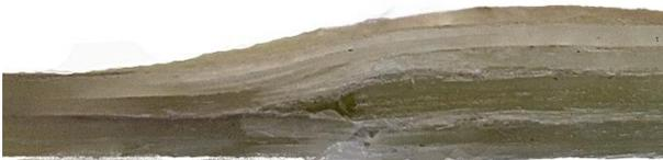
No difference with the previous cuts. Still delamination and fibre failure.
