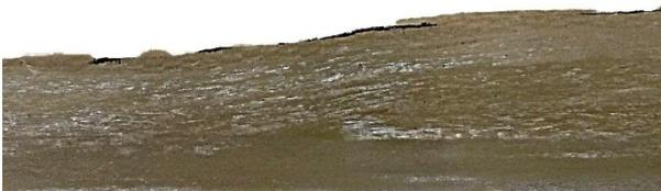
Cut performed at the very beginning of the crack front but damage is not visible yet.
