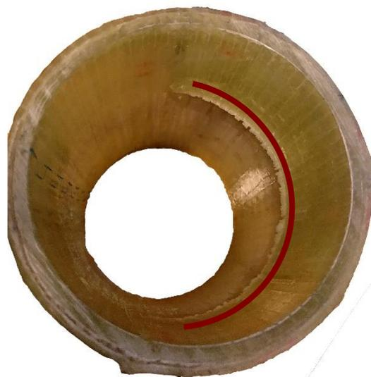
*Figure D.2. The crack front occupies the half of the cylinder under higher pressure.*
