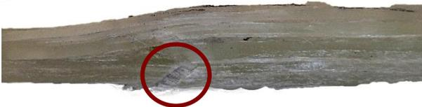
Delamination at the upper layers seem to be less abrupt. Fibres at the bottom part failed forming a kink band due to shear micro buckling.
