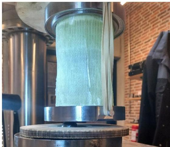
*Figure B.2. Steel ball that concentrate the load to one point.*
