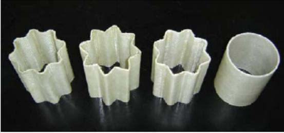
Figure 2: Corrugated profiles tested by Abdewi [4].
