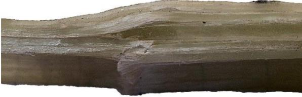
Here the highest damage was expected as this cut was done at the point with higher stress. Delamination is visible at the upper layers of the ply drop as well as fibre failure at the bottom part.
