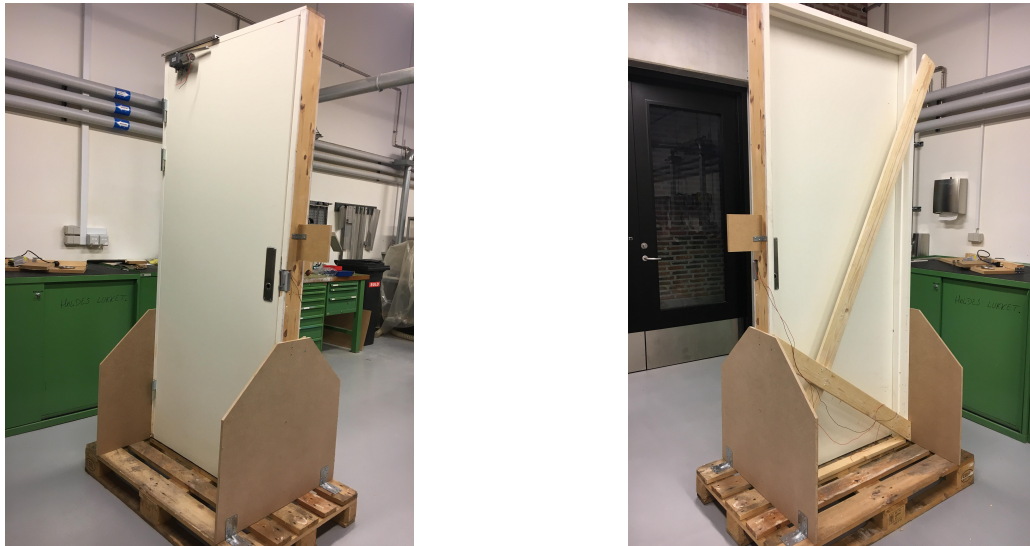
Figure 3.2. Front of our home made door setup Figure 3.3. Back of our home made door setup
