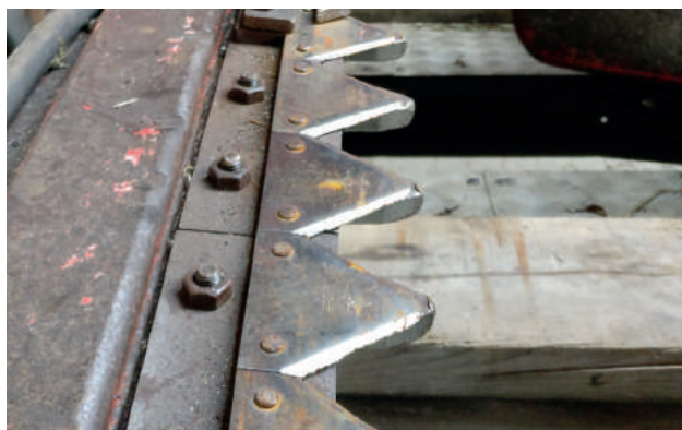
Ill. 2.18 The teeth on the weed cutting boat cutter
