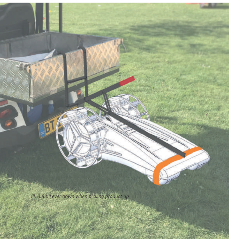
Ill. 1.83. Lever down when picking product up
