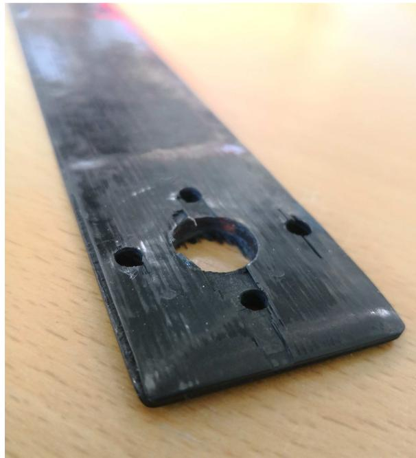
**Figure 7.6:** *Surface of sample after drilling holes.*
