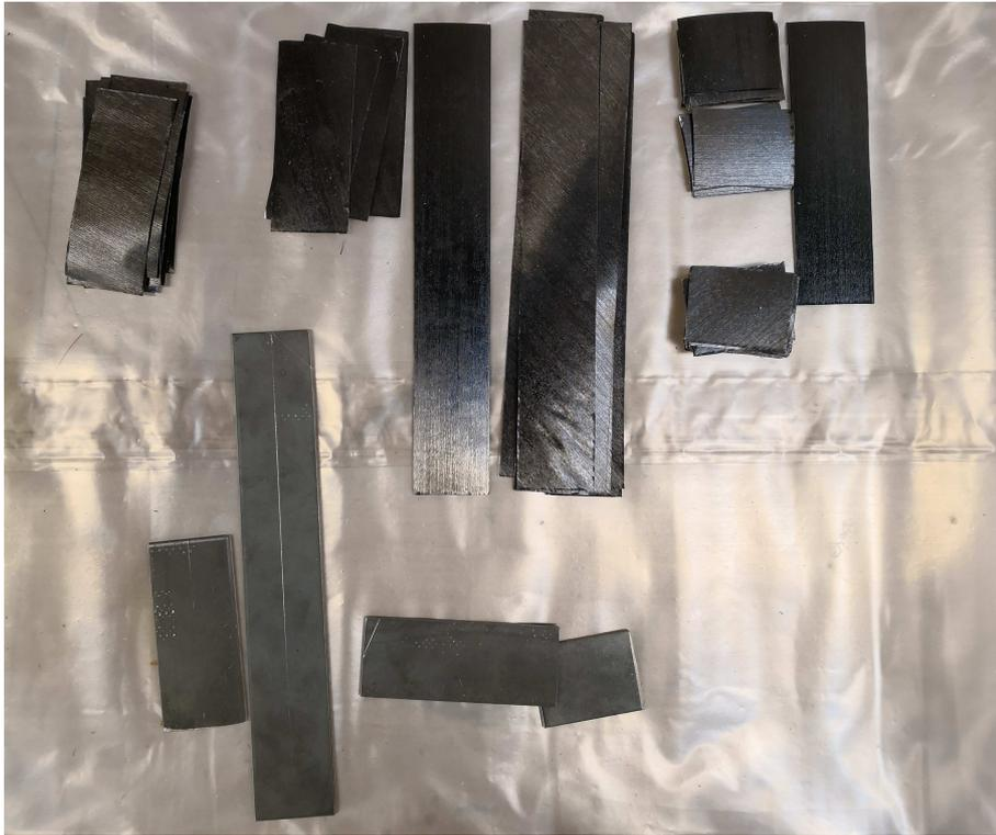
**Figure 6.1:** An example of carbon fibre prepreg plies cut in in several sizes with fibres oriented in  $0^\circ, \pm 20^\circ, \pm 45^\circ, \pm 70^\circ,$  and  $90^\circ$ .
