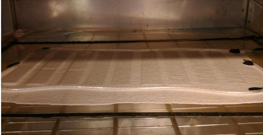
**Figure 7.5:** Vacuum bag including samples prepared for curing.
