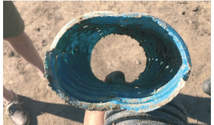
Illustration 69.2 - Deformation of existing drain
