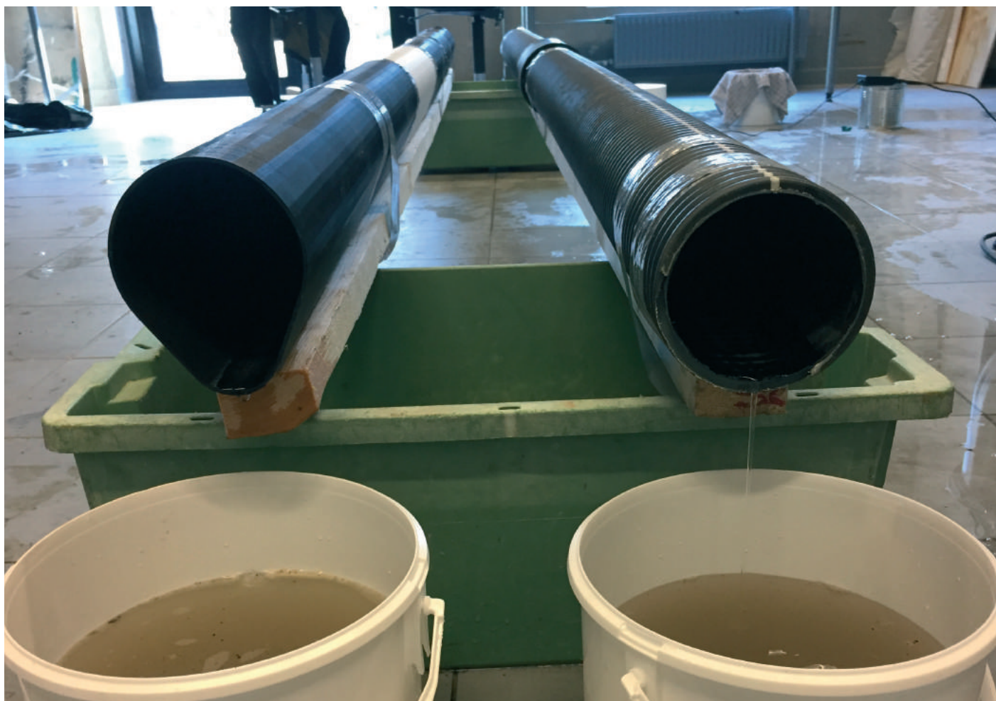
Illustration 63.1 - Test of flow, moving solids
