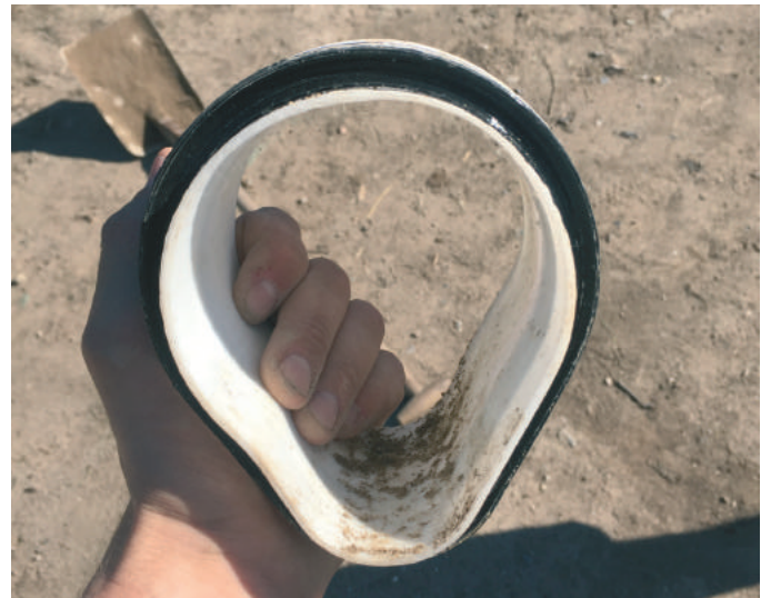
Illustration 69.3 - Deformation of NXD Drain
