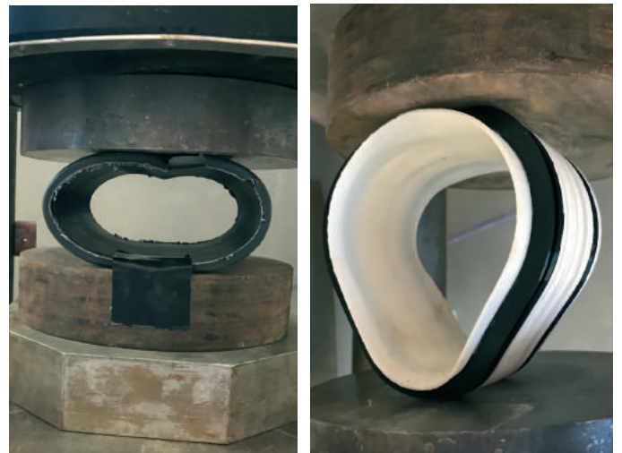
Illustration 69.3 - Deformation of Right: NXD Drain Left: Corrugated drain
