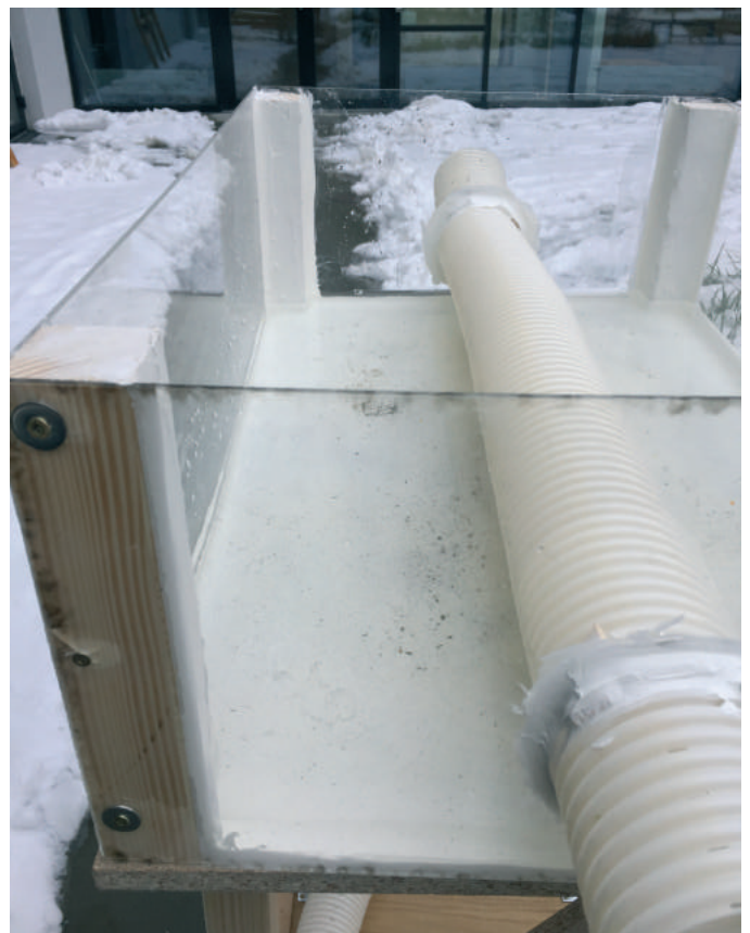
Illustration 60.2 - Water penetration test setup
