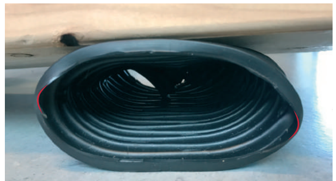
Illustration 37.2 - Deformation of corrugated drain
