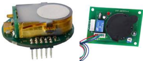
Ill. 05.05: Cozir A CO 2 sensor and photoelectric smoke detector.
