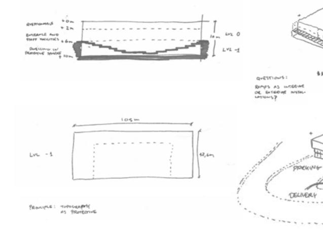
▲ III. 097: A definition of the shape, size and height of the building; approx. 5000 m<sup>2</sup> in plot,10 m tall and spans across two levels. These are defined as IvI. 0 and IvI -1 as most of the lower part of the building is embedded within the ground.
