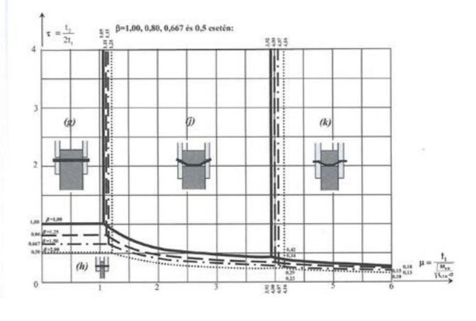
▲ III. 084: Embedment strenght depending on quality of timber and diameter of dowel.<sup>82</sup>
