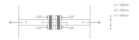
Ill. 087: Static diagram of the truss translating the distribution of forces within the construction of the structure.
