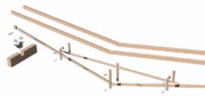
▲ III. 082: Details of the ceiling structure; a tectonic truss that effectively distributes loads into its larger segments via a vertically constructed four-piece element.
