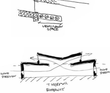
▲ III. 122: Investigations of mixing ventilation principles in the collective and dwelling; having fresh air supply from one side and an outlet on the opposing side. Additionally, the bathroom is naturally granted an outlet.
