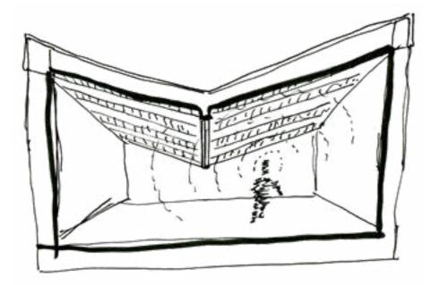
▲ III. 124: Investigations of the acoustic principle of absorption, applying soft surfaces and wooden lamellas in the ceiling of the hall in order to reduce reverberation time and increase intelligibility within.
