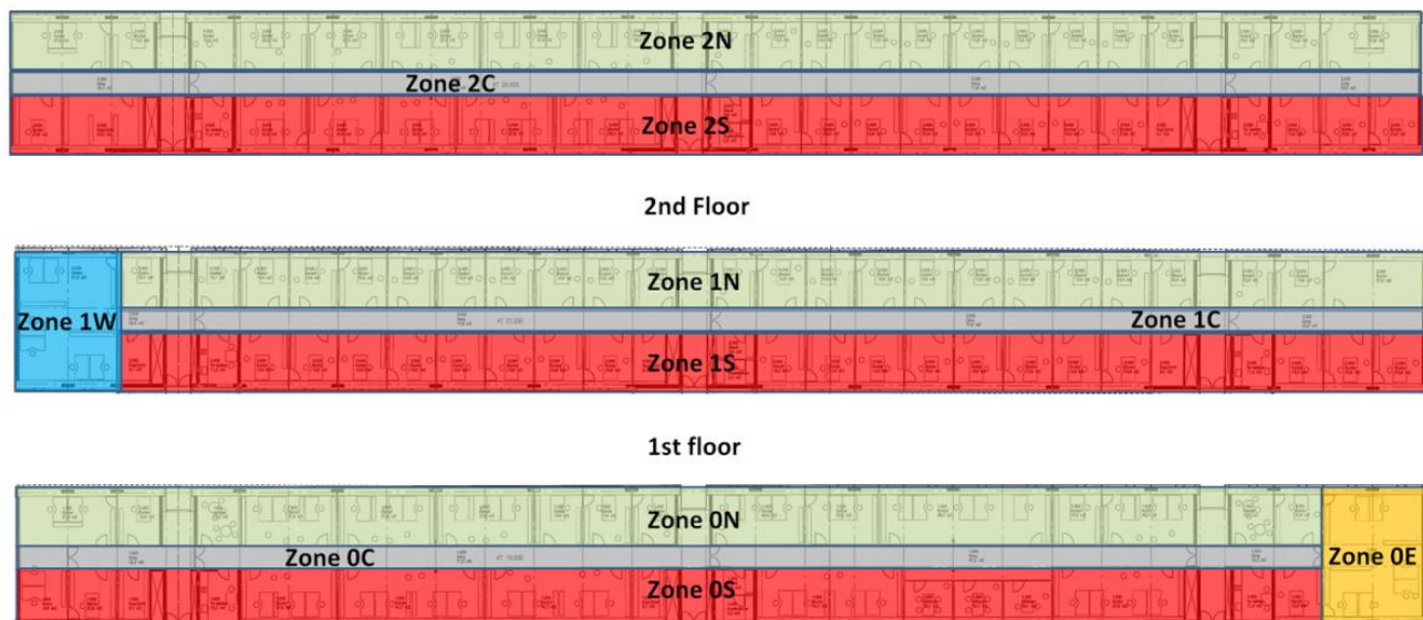
Figure 2 Division of thermal zones in simulated model
