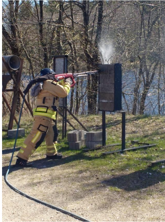
Figure 38 Demonstration of a high-pressure extinguishing system in Borås, Sweden
