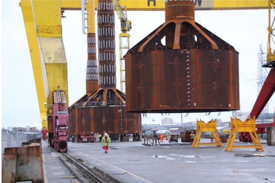
*Figure 2.5.* Monobucket foundations used in the Horns Rev 2 project [Universal-foundations, 2017].
