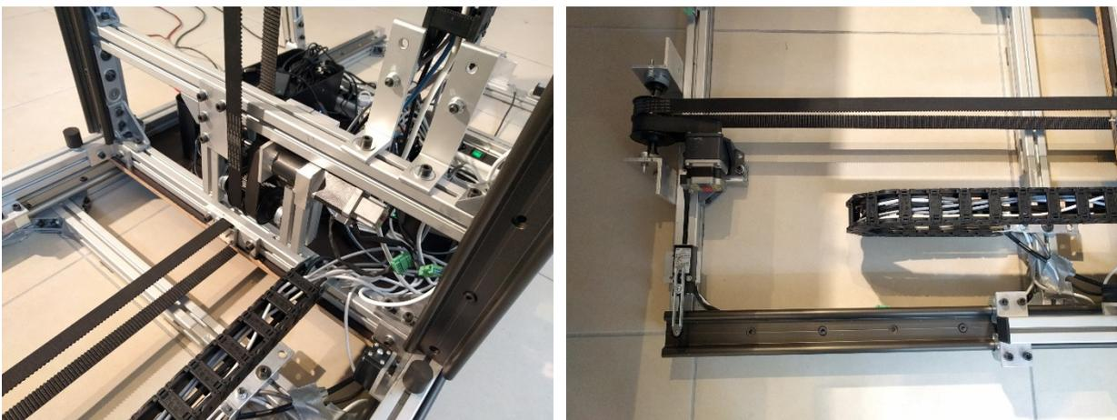
*Figure 38 Close-up showcasing the stepper motors, linear rail and belt driving system*
