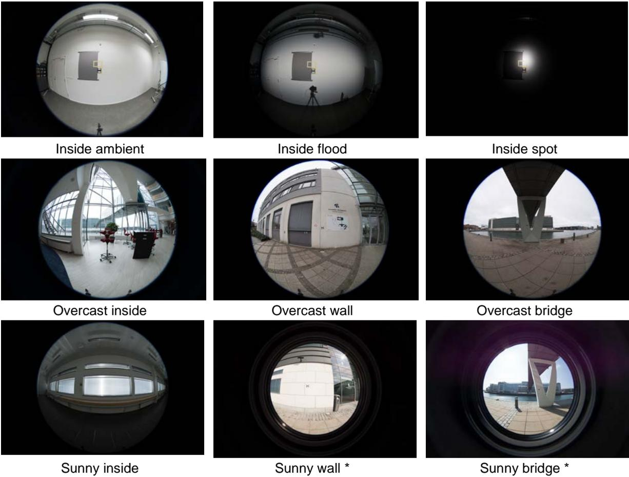
*Figure 22 HDR images for luminance – illuminance calibration tests*
