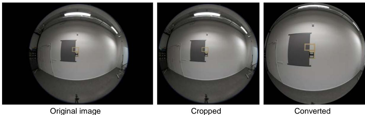
*Figure 18 Image stages for illuminance calibration*
