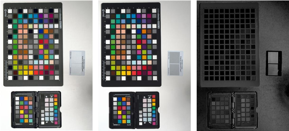
*Figure 33 Unpolarized, polarized and generated specular difference*
