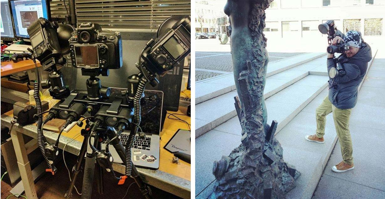
*Figure 35 Portable cross-polarization setup with 1 camera and 2 flash light sources*
