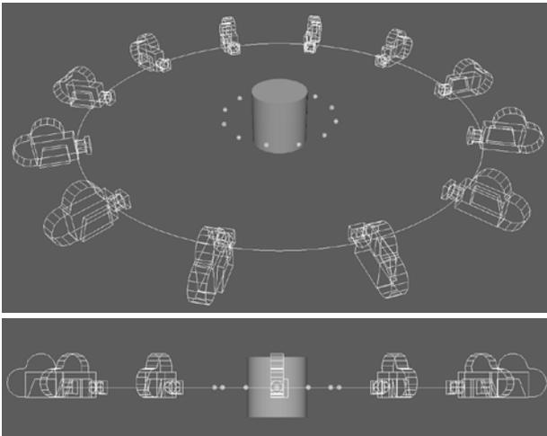
Figure 3 First image set around the whole object
