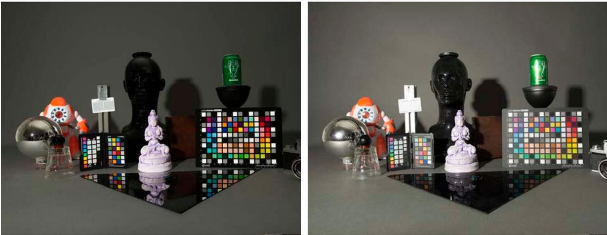
*Figure 34 Cross polarization setup is polarized and unpolarized light*
