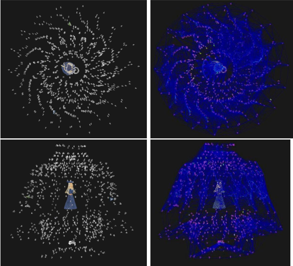
*Figure 41 Top and side view from Reality Capture showcasing intense camera coverage*
