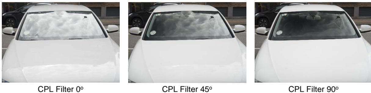
*Figure 32 Circular polarizing filter test*
