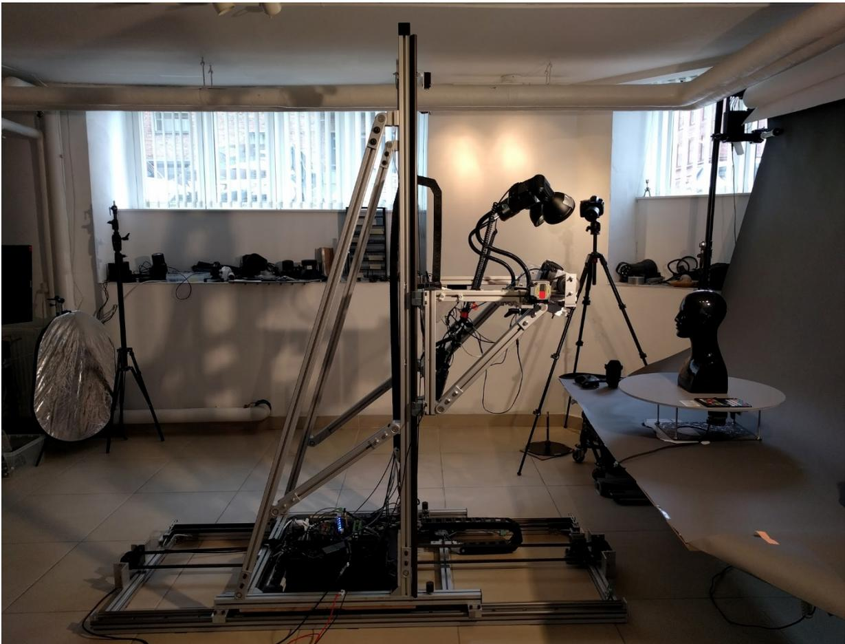
*Figure 37 Side view of the camera rig*
