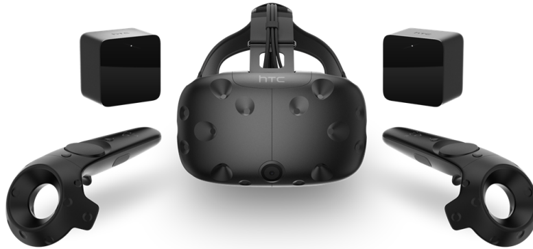
Figure 1.1. An image of the HTC Vive with the vive controllers and the two lighttowers making roomscale possible.
