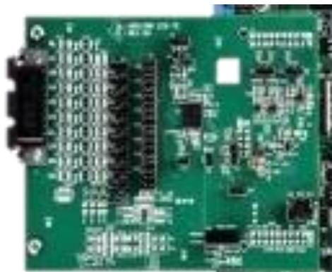
Figure 18 The ADS12398ECGFE-PDK from Texas Instrument used to collect a 3-lead ECG simultaneously with SCG signals.
