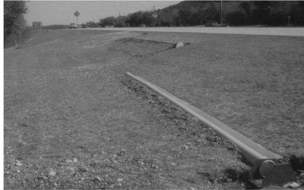
**Figure 3.5:** Sheet flow sampler by Barrett, Kearfott, and Malina (2006).
