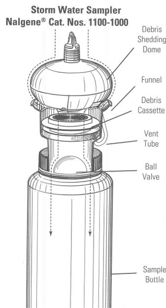
**Figure 3.6:** Nalgene Storm Water Sampler.
