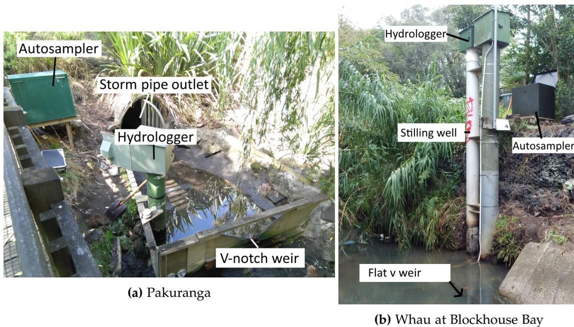
**Figure 4.3:** Overview of the test sites, pointing out the autosampler, storm pipe outlet, hydrologger and the weir.
