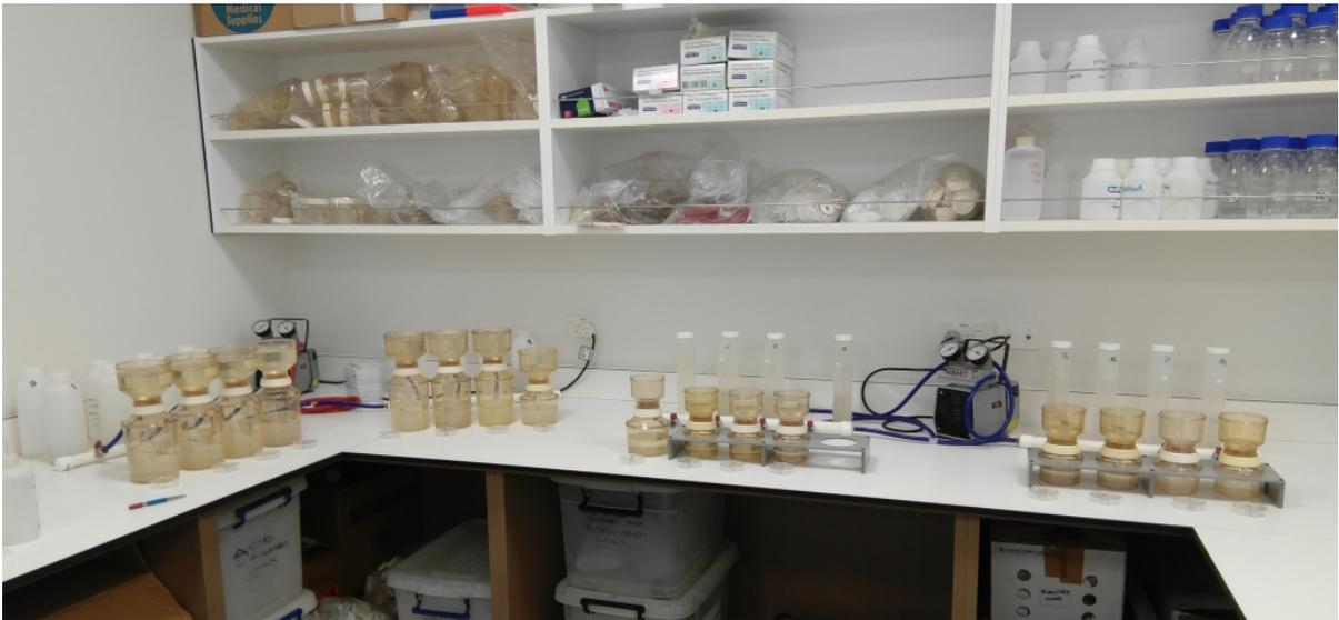
Figure 4.11: SSC analysis setup using vacuum filtration equipment.
