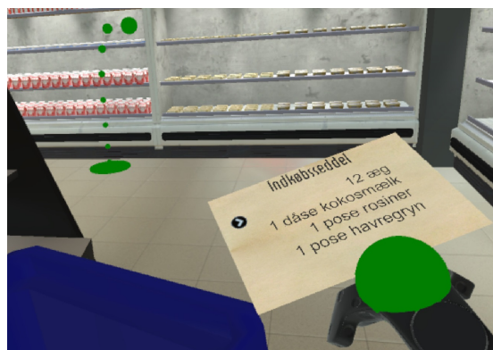
Figure 4.14: The VRTK teleportation utilizes a bezier curve as a pointer to teleport the user to a new location.
