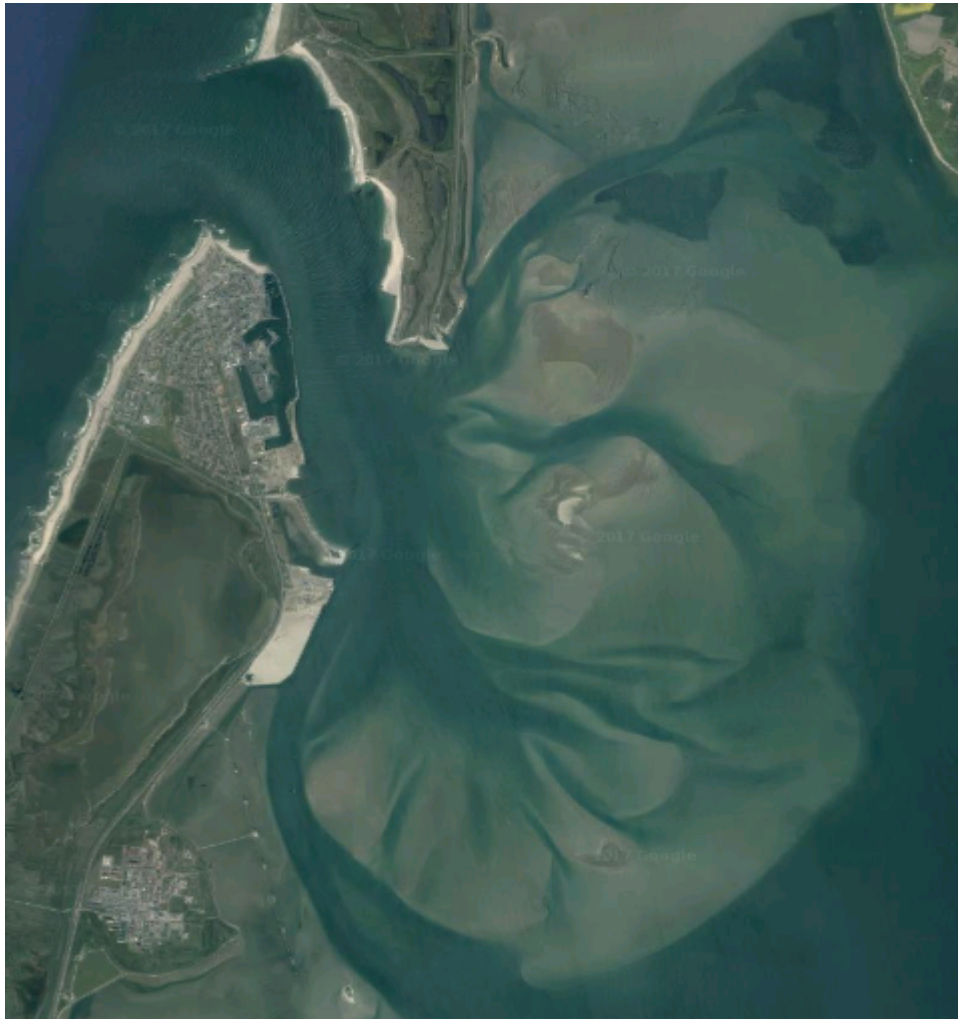
Figure 2.7 Sand banks created by sedimentation from the west coast through Thyborøn Channel [Google, 2017].
