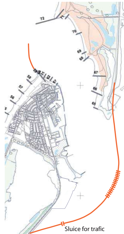
Figure 2.2 Solution proposed by KDI [2012, p. 17]. Construction of dam with sluice and extension of groyne 59.
