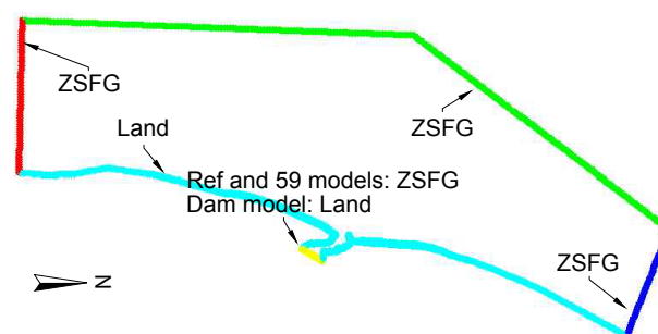
Figure 6.5 Boundary conditions used in the ST module of the Thyborøn model. ZSDG is “Zero sediment flux gradient”.
