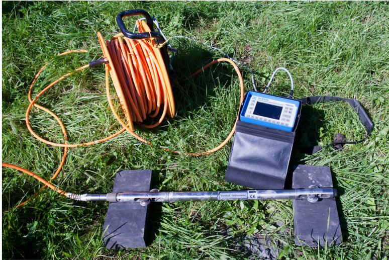
Figure A.177: A typical portable inclinometer.[45]
