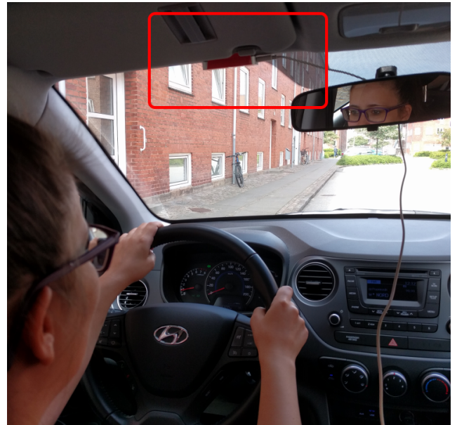
Figure 1. The leap motion placement. The leap motion can capture both hands and a large part of the area of interest.
