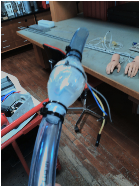
Figure 6.10: Enclosure created for the temperature & humidity sensor.
