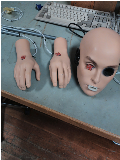
Figure 6.12: Placement of all the luminosity sensors on the manikin's body.
