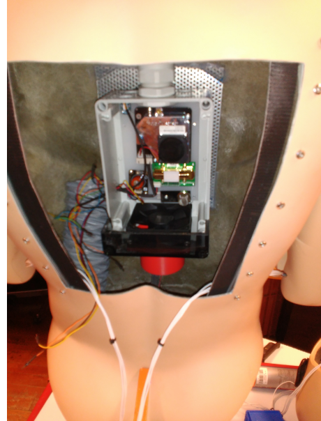
Figure 6.15: The 'air box' mounted inside the torso.
