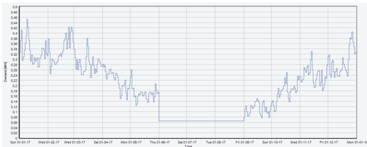
Figure 7.3: Collective heat demand, including heat savings of 20% for Valsted
