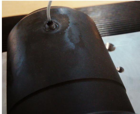
**Figure 5.19:** *A picture showing the transducer glued to the cylinder surface.*
