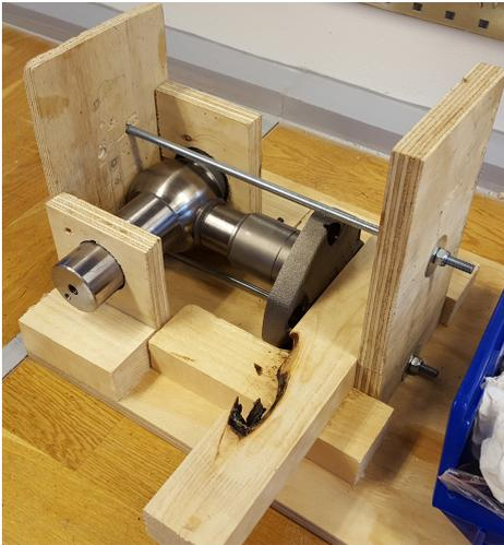
**Figure F.3:** Test setup to measure the largest static friction.
