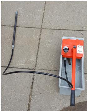
**Figure G.1:** *Picture of the assembled equipment used for the pressure test.*
