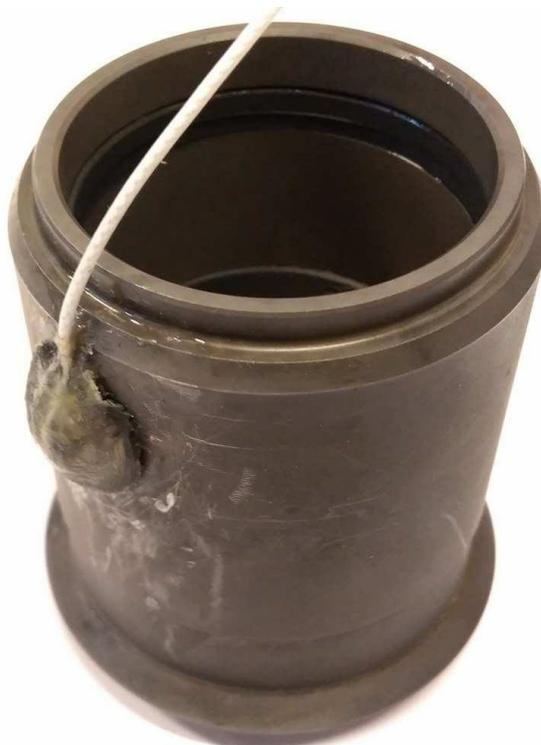
**Figure 5.22:** *Picture of the cured epoxy cast after mold removal.*
