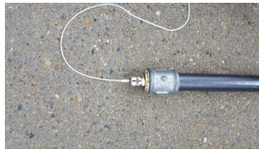
**Figure G.2:** *Close up of the screw coupling used to seal the wires exit and the connector used to assemble the water pipe and screw coupling.*
