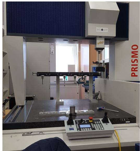
**Figure 6.6:** Coordinate measuring machine used to measure difficult geometries on the telescopic cylinder.
