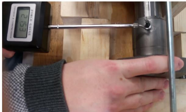
**Figure F.4:** Picture of test where the largest static friction has been measured and the cylinder has moved.
