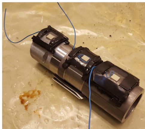
**Figure 5.17:** *Epoxy adhesion and wire clamping tests with different surface roughness.*
