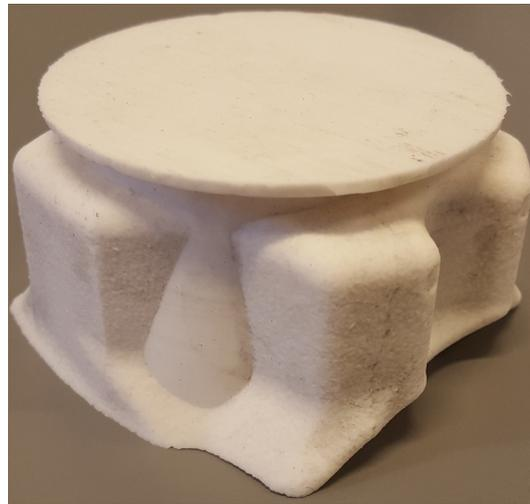
**Figure 6.3:** Silicone cast of part of the motor cavity, which makes it possible to accurately estimate the internal features of the motor cavity.
