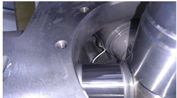
**Figure 7.2:** *The telescopic cylinder with the mounted transducer is shown. The transducer wire is seen exiting the motor through the flushing connector.*
