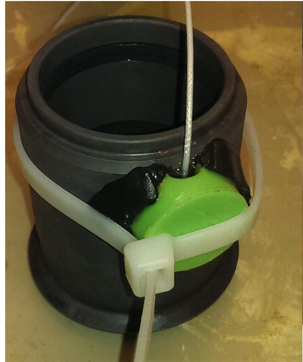
**Figure 5.21:** *Picture showing the mold fastened to the cylinder, with tape and glue applied.*
