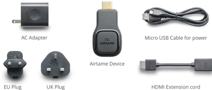
Fig.4 Overview of the Airtame components and features (Airtame, 2017, online)
