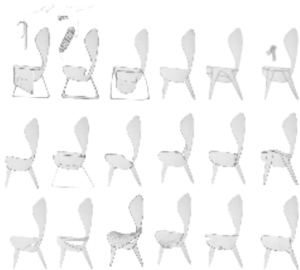
Figure 87. Quick sketches for how armrest could look like and how legs could be an integrated part of it.
