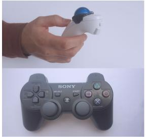
*Ill.* **55**: Trackball controller and Play station 3 controller to simulate an analogue stick
