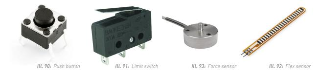
To find and determine the right type of actuation for the product, the four candidates have been assessed on their potential within: adjustment options for clicking position, feedback, size, and placement options (*III. 94*).
