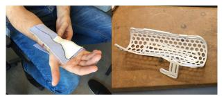
Ill. 67: Left: Cutting out cloth template. Right: 3D printed brace
