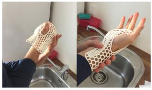
Ill. 65: Testing thermoforming of 3D printed brace
