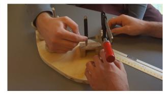
Ill. 97: Finger resistance test setup
