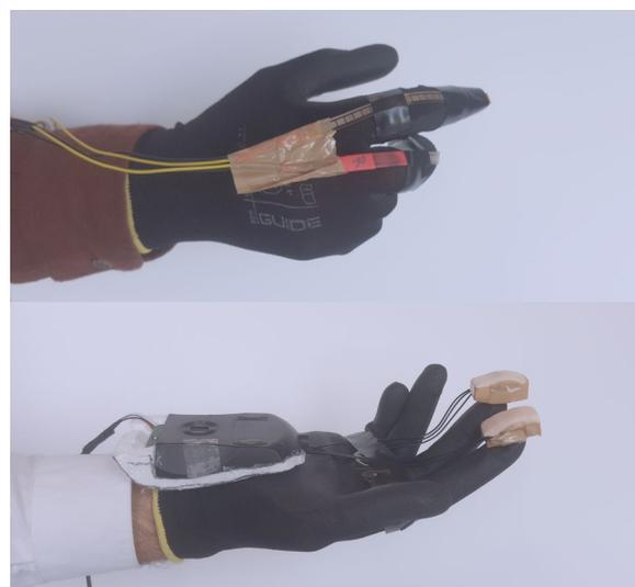
Ill. 56: Flex sensor glove and push button glove. Both with optical sensor from disassembled mouse
