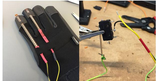
Ill. 72: Left: Flex sensors. Right: Connecting switches
