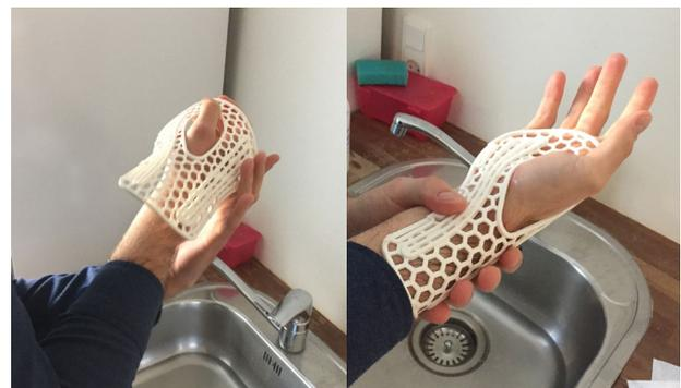
Ill. 65: Testing thermoforming of 3D printed brace
