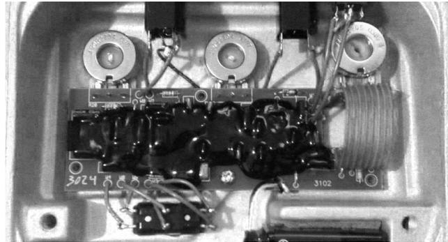
**Figure 2.4:** Picture showing the black epoxy - a measure taken to prevent 'cloners' from copying the effect pedal circuit. *Image source: <https://soundvacuum.wordpress.com/>*
