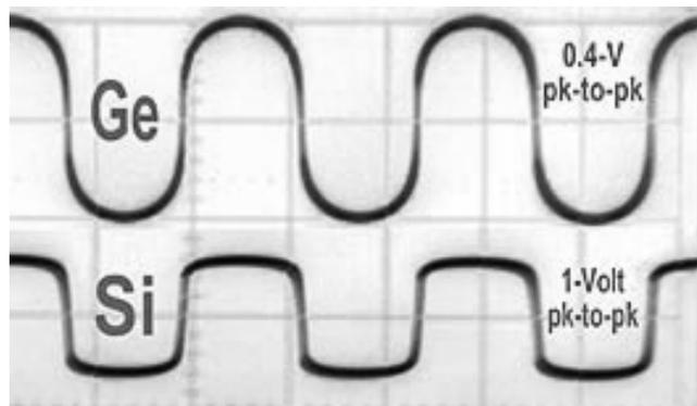
**Figure 3.9:** The different clipping characteristics of the softer clipping germanium (top) and the harder clipping silicon (bottom) as seen on an oscilloscope. *Image source: <http://www.mixonline.com/news/profiles/guitar-distortion/365765>.*
