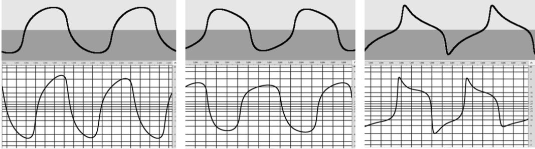
Bypass 'Tone' filtering at min., med. and max. settings. Top: simulated. Bottom: Recordings.
