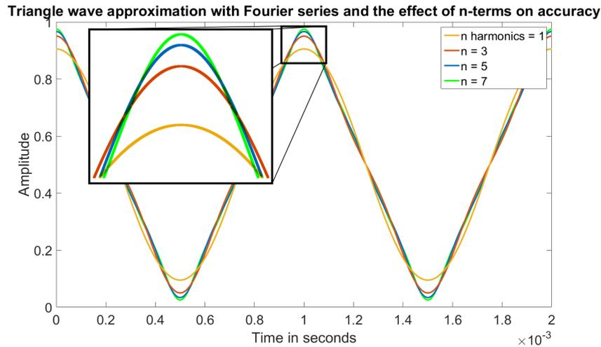
**Figure 2.7:** Matlab plot of how the number of 'N-included' harmonics affect the accuracy of the Fourier series of a triangle wave.
