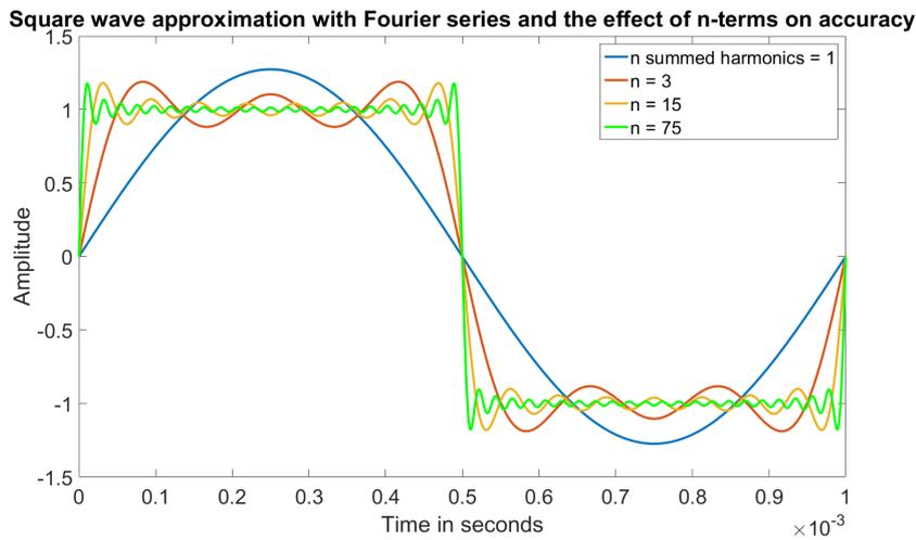
**Figure 2.6:** Matlab plot of how the number of 'N-included' harmonics affect the accuracy of the Fourier series of a square wave.
