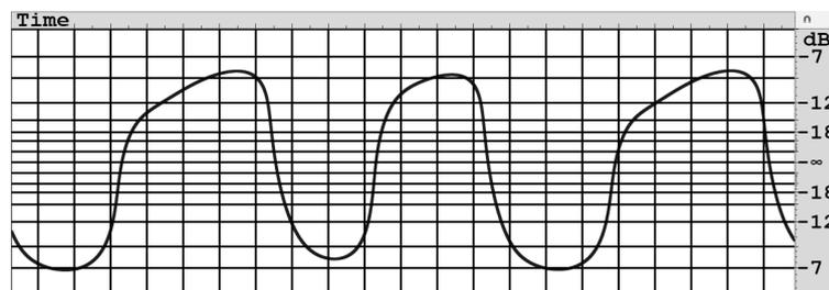
**Figure 3.10:** Example of the asymmetrical germanium diode clipping. The recording is of an open  $D_2$  played with the 'Hi' setting and all knobs set to 12 O'clock. The positive half-wave cycle is more aggressively clipped than the negative wave cycle.
