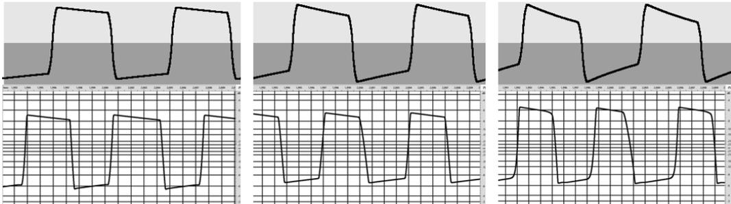
Silicon 'Tone' filtering at min., med. and max. settings. Top: simulated. Bottom: Recordings.
