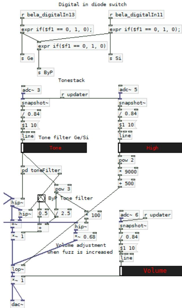
Figure 4.7: The implementation of the tonestack and output segment in Pure Data.
