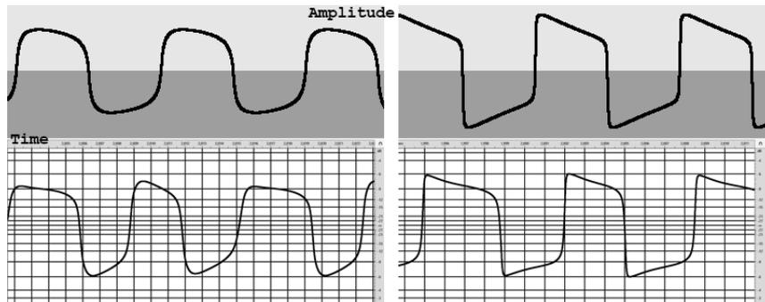
**Figure 4.6:** Top left: Simulated version of the 'Silicon' recording with fuzz at min. setting. Top right: Simulated with fuzz at max. Bottom left: Recording with fuzz at 8 O'clock setting. Bottom right: Recording at 4 O'clock setting.
