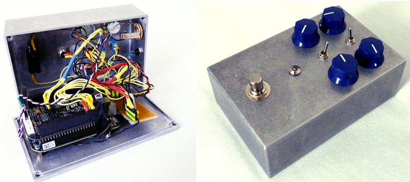
**Figure 4.9:** Left: The internal of the created pedal with microcontroller, wiring to the switches, potentiometers, diode, DC source connection and audio in/out. Right: The assembled pedal box.
