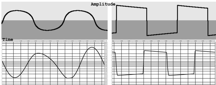
**Figure 4.5:** Top left: Simulated version of the 'Bypass' recording with fuzz at min. setting. Top right: Simulated with fuzz at max. Bottom left: Recording with fuzz at 8 O'clock setting. Bottom right: Recording at 4 O'clock setting.
