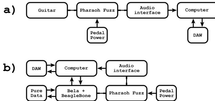
**Figure 3.2:** Setups used for recording analysis signals. a) Setup used to record notes played on various pedal configurations. b) Setup used to generate white noise, which was fed to the pedal to get frequency responses for various pedal configurations.
