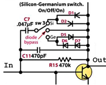
**Figure 1.4:** The selectable clipping diodes of the second clipping stage. The components are connected in feedback loops, which saturate the sound. A high signal level will result in more saturation because of the increased clipping. *Original image source: <http://www.bigmuffpage.com>*
