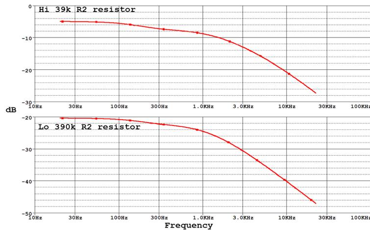
**Figure 3.4:** SPICE simulation of the input segment. The 'Fuzz' knob potentiometer (R7 in *figure 3.3*) is set to low resistance at 1 Ohm (high signal strength). The top graph is the 'Hi' setting, bottom is the 'Lo' setting. Note the different intervals along the y-axes.
