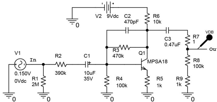
**Figure 3.3:** The input segment of the Pharaoh fuzz. The R2 resistor is the 'Lp' setting of the 'Hi-Lo' switch. R7 is the potentiometer connected to the 'Fuzz' knob, here set at minimum resistance. Probing for the filtering characteristics was performed at the output of the input segment.
