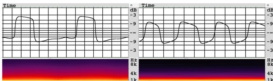
**Figure 3.5:** Two waveforms and spectrograms from recordings of D-notes played open at the same settings, all knobs at 12 O'Clock, with silicon diodes at about the same instance after the attack: 2 seconds in. The depicted signal in the left window was recorded with the 'Hi' configuration. The right was recorded with the 'Lo' configuration.
