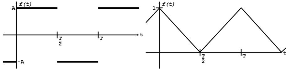
Figure 2.5: Sketches of wave functions. Left: Square wave function. Right: Triangle wave function.
