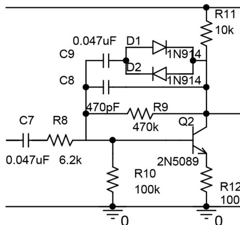
**Figure 3.6:** Section of the SPICE modeled first clipping segment. The top input is connected to a 9V DC source.
