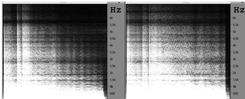
**Figure 5.2:** Spectrograms of a power cord played twice followed by an open strum of the same strings. Left: The emulation pedal. Right: The pharaoh. Both recordings are about 14 sec. in length, note the difference in sustain, which can be seen as more brightness along the X-axis.
