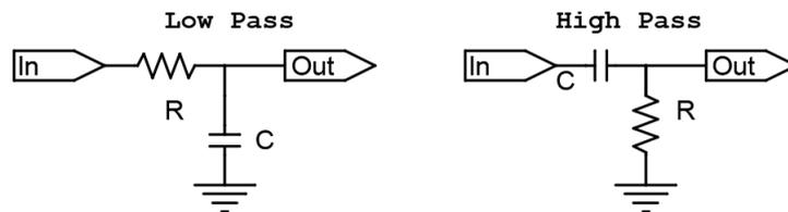
**Figure 3.14:** The two RC circuit configurations for the first order low-pass filter (left), and first order high-pass filter (right).
