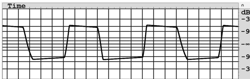
**Figure 3.7:** Recording showing the waveform of an open  $D_2$  note with all knobs set to 12 O'clock, 'Hi', and second clipping segment bypassed. The illustrated section is approximately 1.5 sec. after the strum.
