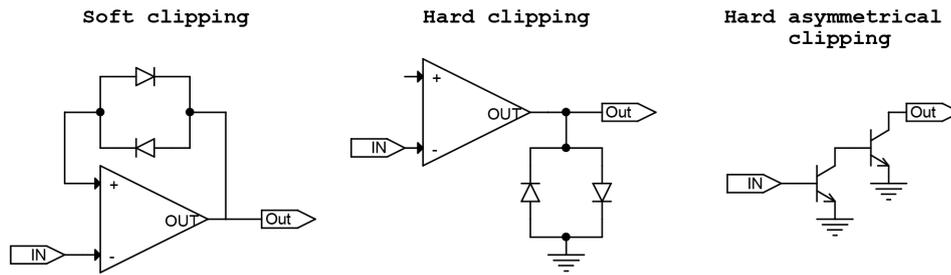
**Figure 1.1:** Examples of how different types of signal clipping can be achieved in electronic circuits.
