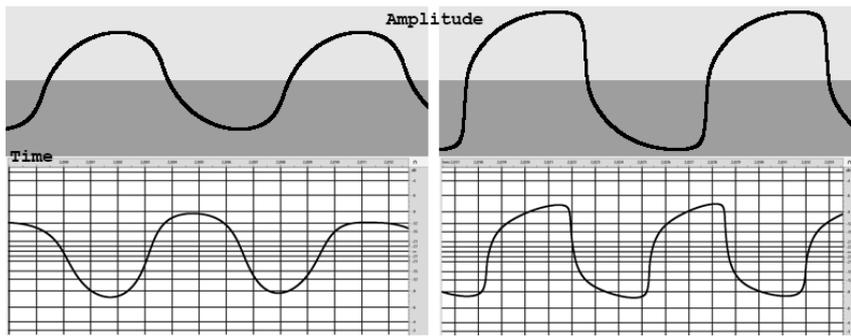
**Figure 4.4:** Top left: Simulated version of the germanium recording with fuzz at min. setting. Top right: Simulated with fuzz at max. Bottom left: Recording with fuzz at 8 O'Clock setting. Bottom right: Recording at 4 O'Clock setting.
