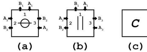
**Figure 2.3:** Graphical representation of three WDF components, including two adaptors and a one-port element. Three-port serial (a), and three-port parallel (b). (c) represents a one-port capacitor.
