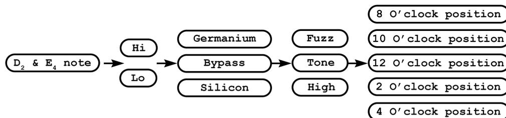
**Figure 3.1:** Overview of the recorded analysis signals. 90 signals were recordings of open  $D_2$  notes and the same number of  $E_4$  notes. The recordings were sampled in the 'Hi' and 'Lo' configuration for all three clipping settings with the 'Fuzz', 'Tone' and 'High' knobs in five different positions.
