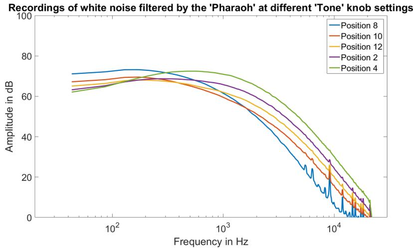
**Figure 3.12:** Frequency response of the five recordings from the different 'Tone' knob positions.
