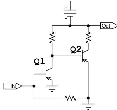
**Figure 2.2:** Simplified transistor circuit of the Fuzz Face intended for analysis.
