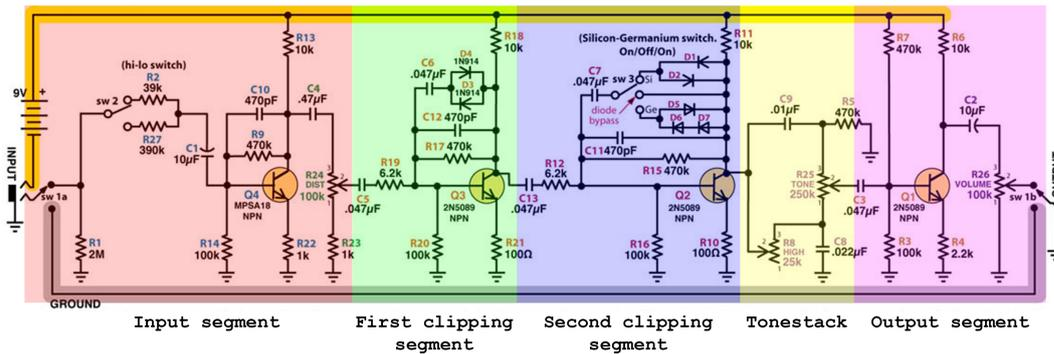
**Figure 1.3:** Black Arts Toneworks Pharaoh Fuzz circuit schematic, see *Appendix A* for a larger representation, with the different segments highlighted. *Original image source:* <http://www.bigmuffpage.com>
