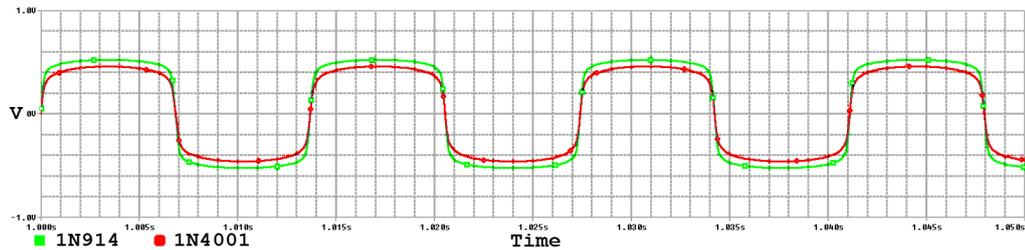
**Figure 3.11:** SPICE simulated waveform of the 1N914 silicon diode of the first clipping segment and the 1N4001 silicon diode of the second clipping segment.
