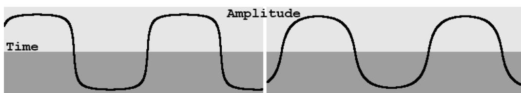
Figure 4.2: Bela simulations of silicon diodes: Left: 1N914, Right: 1N4001.
