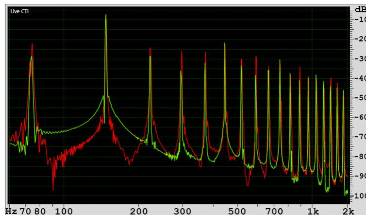
**Figure 4.8:** The frequency spectrum from recordings of two open  $D_2$  notes at played at two different 'High' settings. Green played at 8 o'clock setting. Red played at 4 o'clock setting.
