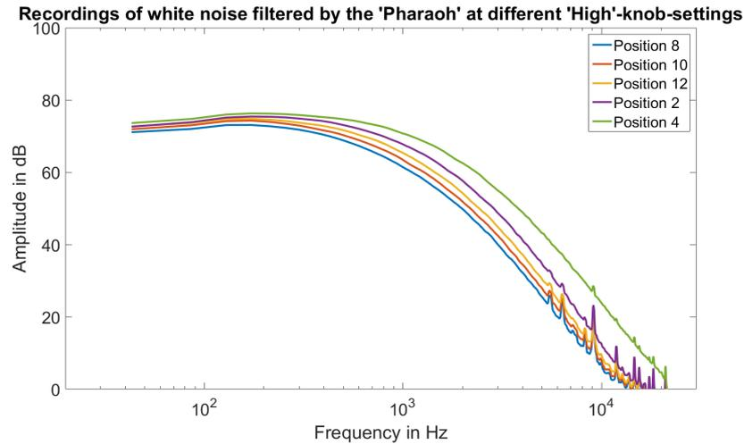
**Figure 3.13:** Frequency response of the five recordings from the different 'High' knob positions.
