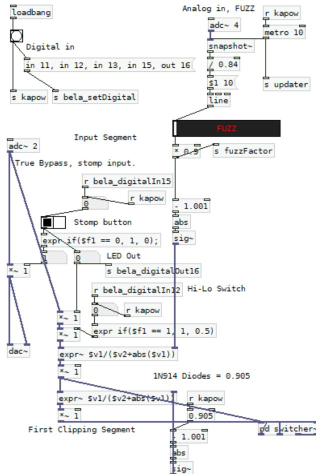
**Figure 4.1:** The input and first clipping segment of the fuzz pedal as it was implemented in Pure Data. Also included in this part of the patch are examples of how to deal with analog and digital I/O communication with the bela cape.
