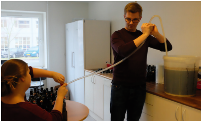
#63.1 Pumping beer into bottles, keeping the inlet above the yeast
