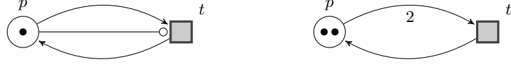
(a) A Petri net illustrating why inhibitor arcs does not work in the siphon-trap property. (b) A Petri net illustrating why arc weights does not work in the siphon-trap property.
