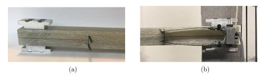
Figure 5.2: (a) Moment arms grips. (b) Clip gauge mounted in the test set up.
