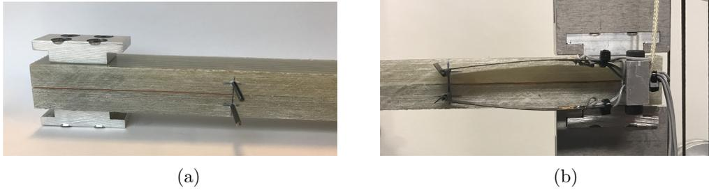
Figure 5.2: (a) Moment arms grips. (b) Clip gauge mounted in the test set up.
