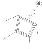
Fig. 5.19: Integrated solar-panels in the window frame
