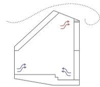
Fig. 5.20: Natural ventilation by thermal buoyancy
