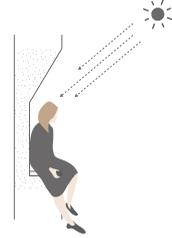
Fig. 5.14: Integrated concrete bench heated by the sun.
