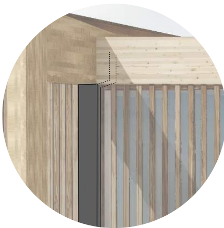
Draining system as a part of the facade expression.
