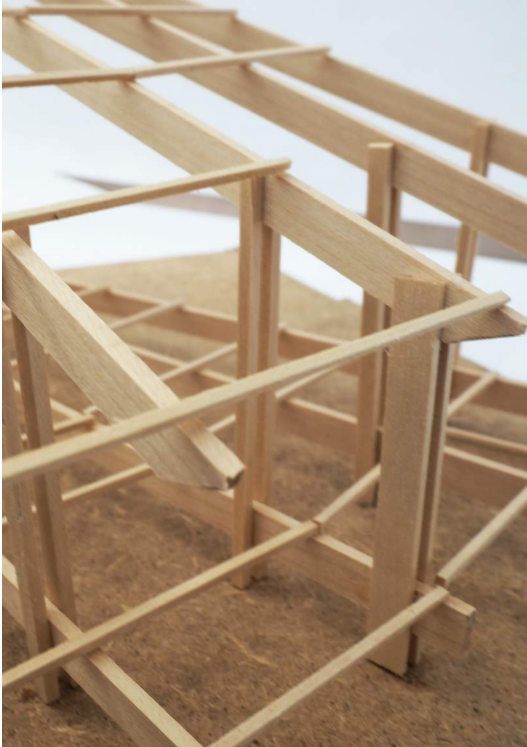
ill. 5.25 | Structural process model of a frame structure
