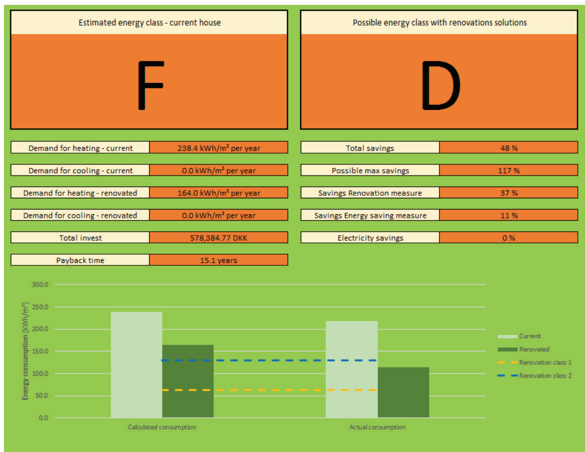
Figure 5.15 Final results illustrating energy consumption and energy mark
