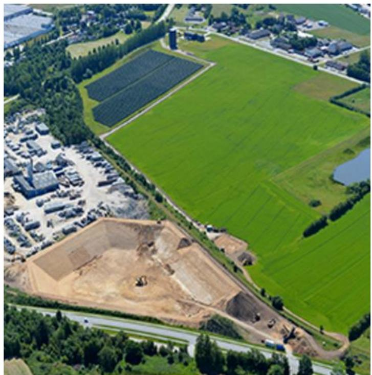
Figure 14 PTES Vojens, Denmark Source [ The world's largest solar heating plant to be established in Vojens, Denmark]
