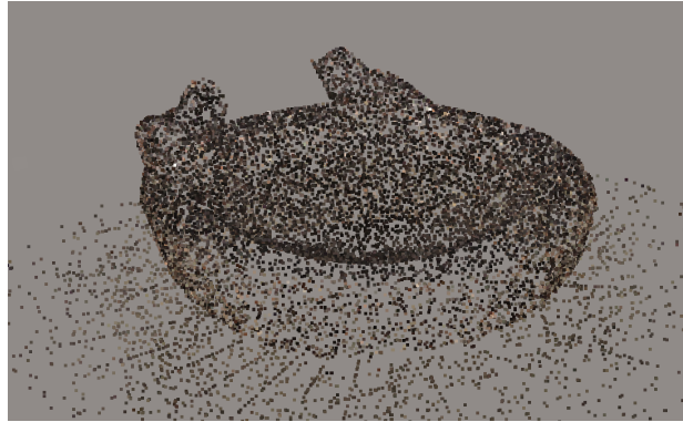
Figure B.1: The resulting pointcloud. Each square is a matched and triangulated feature.
