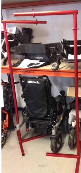
Figure 7: Custom-made adjustable microsoft kinect camera tripods.
