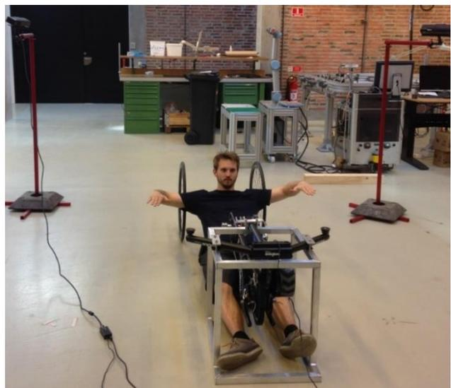
Figure 2 : Experimental setup with handbike connected to home trainer mounted in a customize upside-down frame. The Microsoft Kinect cameras for obtaining kinematic data are located on top of the red camera tripods.
