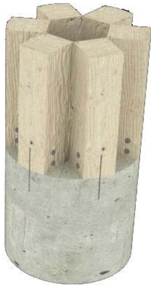
III.218 Wood beams rest on concrete with steel joint
