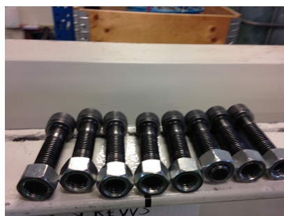
Figure A.35: Black bolts used for fixing the piston in the middle position.
