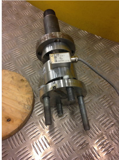
Figure A.36: Head attached to the hydraulic piston controlled by force.
