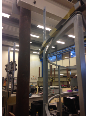
Figure A.7: Pipe controlling the gradient.
