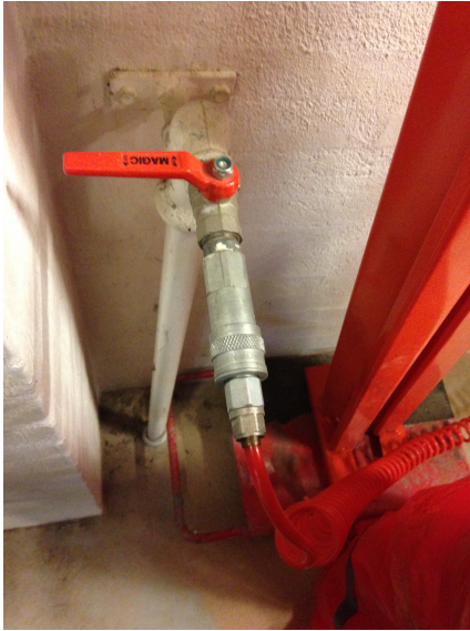
Figure A.44: Control system of the vacuum.
