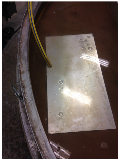
Figure A.32: Metallic plate for filling the container with water during the test.
