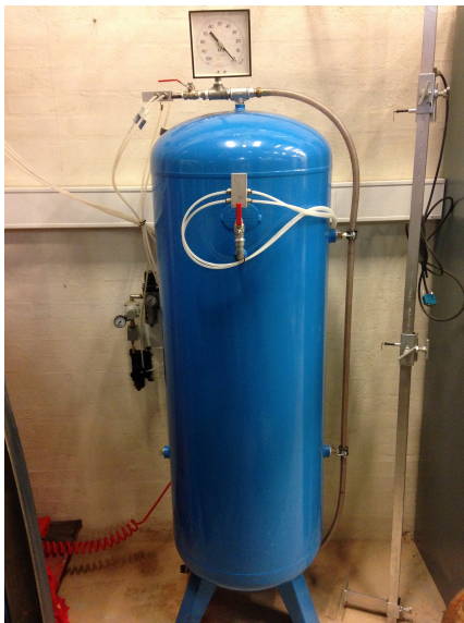
Figure A.43: Connection of the pipes from the vacuum, with the valves for suction.
