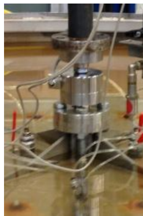
Figure A.39: Connection of the bucket with the force head.
