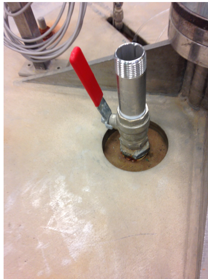
Figure A.49: Connection of the bucket with the hose.
