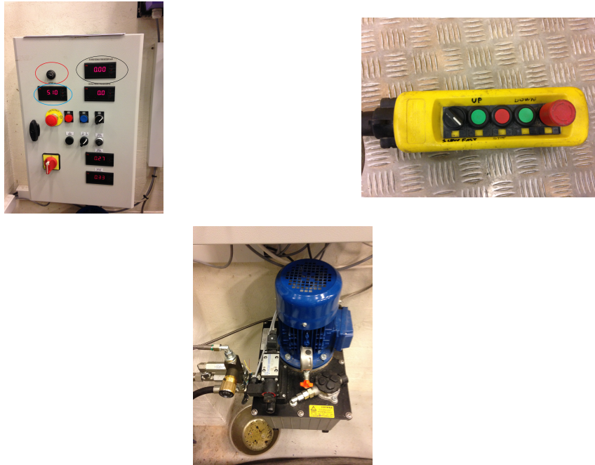
Figure A.18: Control panel, yellow controller and the pump of the hydraulic piston.
