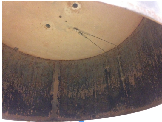
Figure A.45: Inside of the bucket (pressure transducer under the lid, PP7).
