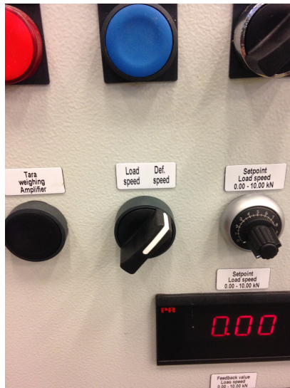
Figure A.37: Control panel switch from displacement to force.
