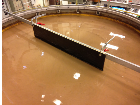
Figure A.11: Bar used for level the soil surface.
