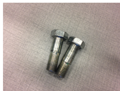
(b) Small bolts used for connecting the head with the CPT rod.
