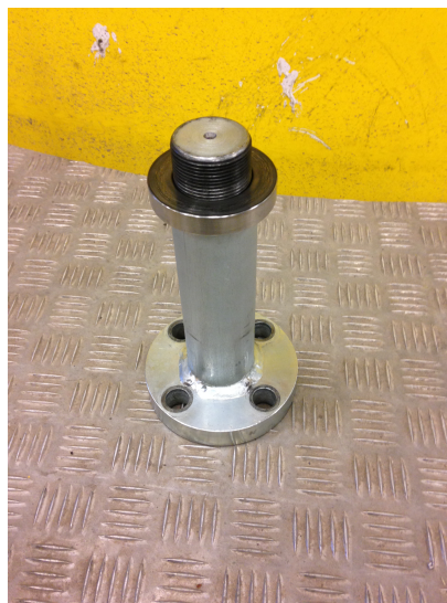
Figure A.47: Head of the piston used for force installation.
