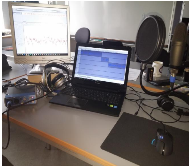
Figure 31. The audio recording setup with computer, external audio card and microphone.
