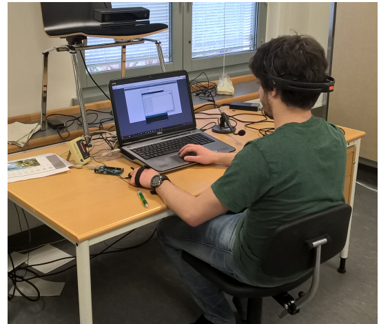
Figure 2. An example of the sensor setup used on the test participants. As he uses his right hand to control the trackpad, the Thoughtstream and Pulse Sensor are attached to his left palm and left index finger respectively. Furthermore, the Kinect can be seen above the monitor aimed at the test participants face. The test participant can also be seen wearing the Epoc device on his head.
