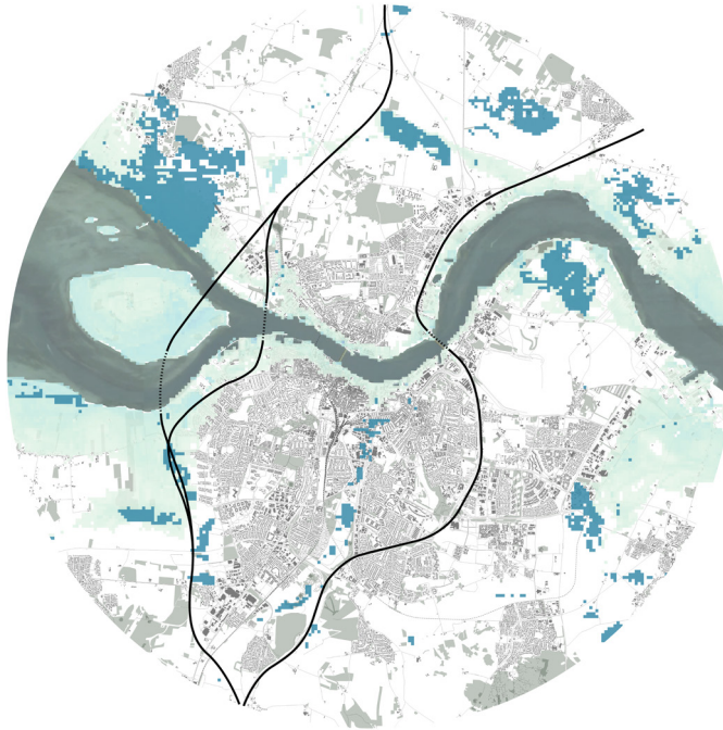
46. CLIMATE CHANGES WITH A 20 YEAR EVENT IN 2100 A rise of 0,98 meters in the year 2100 and a 20 year event with a rise of an extra 1,3 meters (green/light blue) alongside a 40 cm rise in smaller watercourses and streams (blue)
