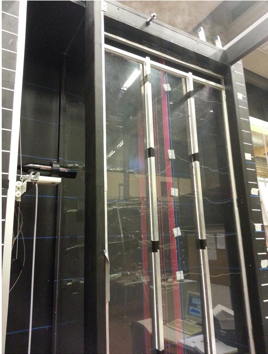
*Figure C.3.* LDA probe placement
