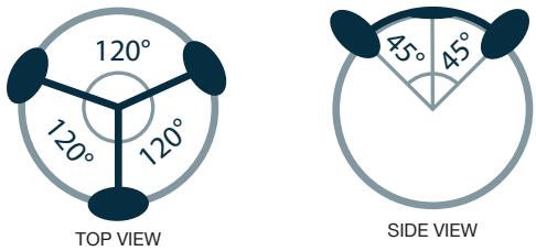
Illu. 65 - Principle structure of omni wheel placement..
