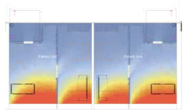
III. 130: Radiation test of Iteration 1
