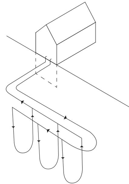
*ill. 042-B: Brine to water system producing sustainable heat by using the passive heat storage with the ground.*
