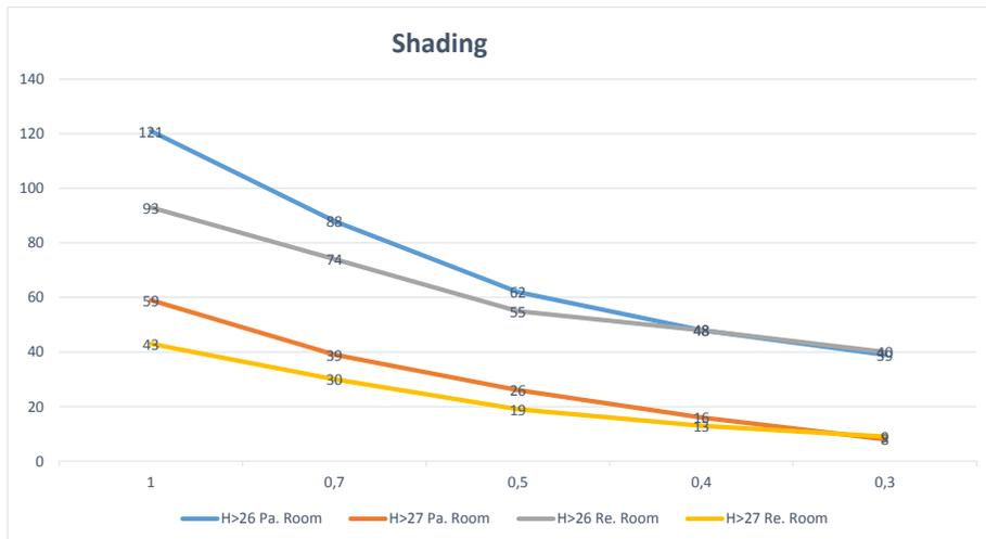
Ill. 209: Bsim analysis showing shading factor compared to the amount of hours above 26 and 27 degrees for patient unit facing west
