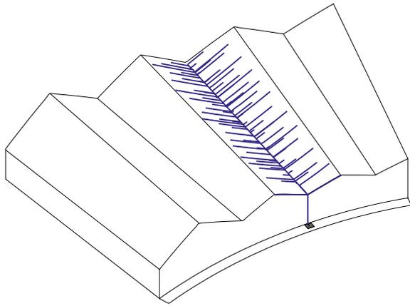
Ill. 187: Diagram illustrating how rain travels along the roof tops
