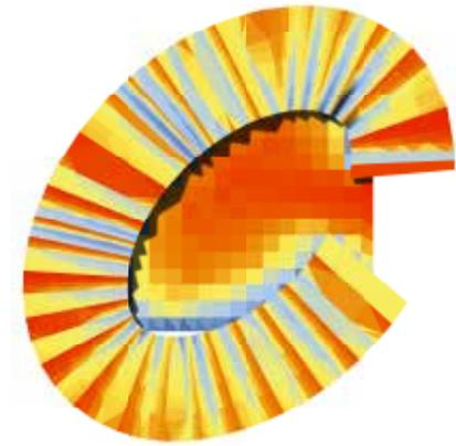
ill. 114: Iteration 7 solar analysis from 100 to 1200 kW/h m<sup>2</sup>
