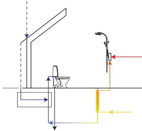
Ill. 188: Diagram showing the utilization of rainwater
