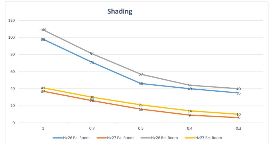
Ill. 210: Bsim analysis showing shading factor compared to the amount of hours above 26 and 27 degrees for the patient units facing south
