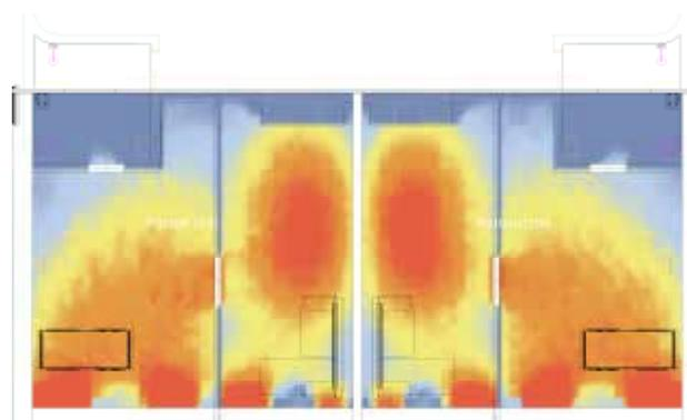
III. 133: daylight test of Iteration 10 with skylight
