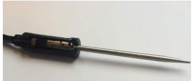
III. 129 - Cut out of the silicone housing the probe
