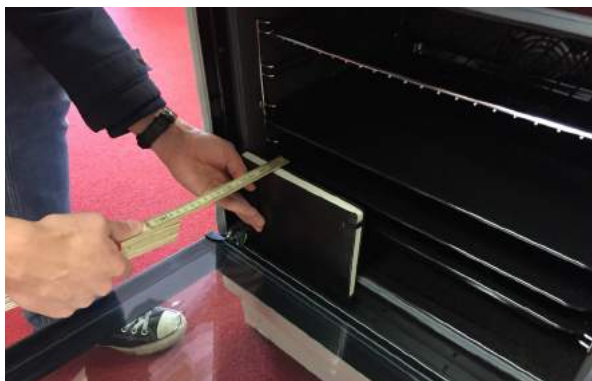
Measuring the distance from the baking plate to the glass door
