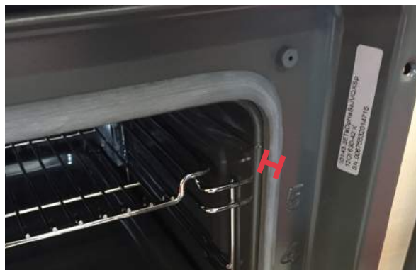
Measuring the size of the rubber sealing
