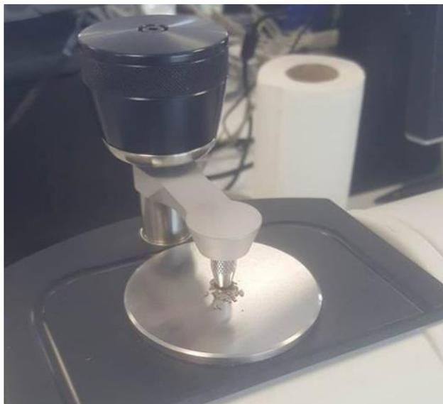
**Figure 41. IR measurement of a geopolymer sample in progress**
