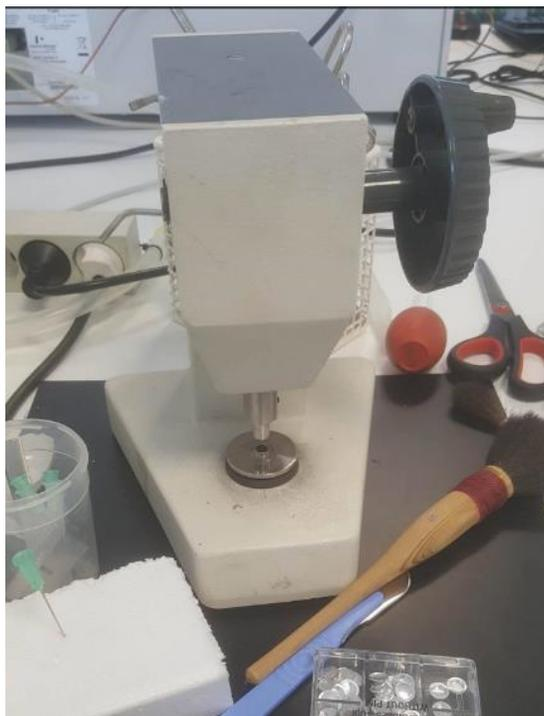
**Figure 58. Press used to seal crucibles**
