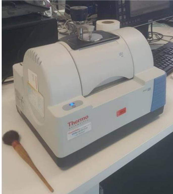
**Figure 40. FTIR-ATR used to measure cement samples**
