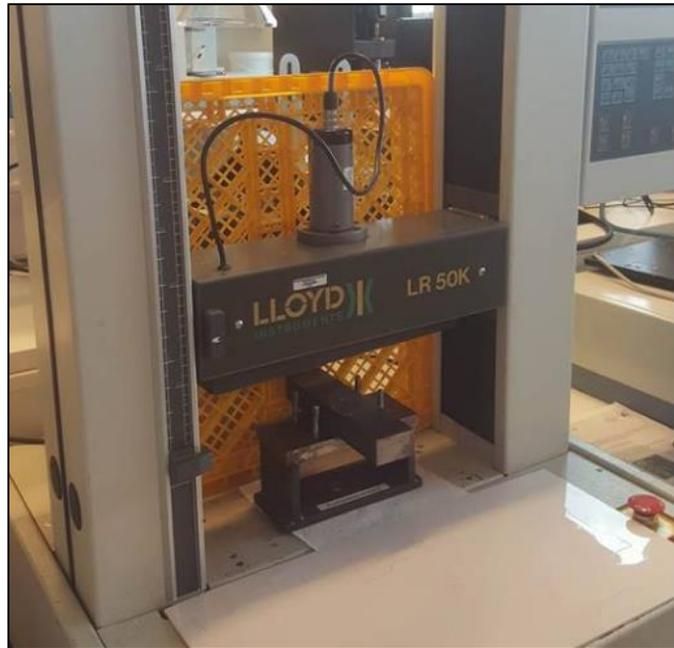
**Figure 76. Compressive machines used for the experiments**
