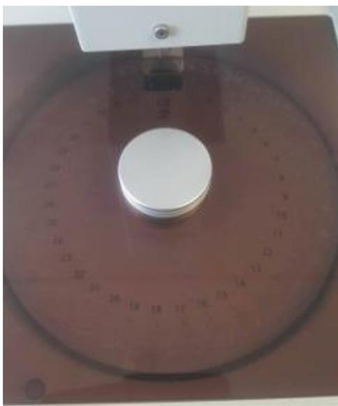
**Figure 59. Sampler plate on the DSC apparatus**
