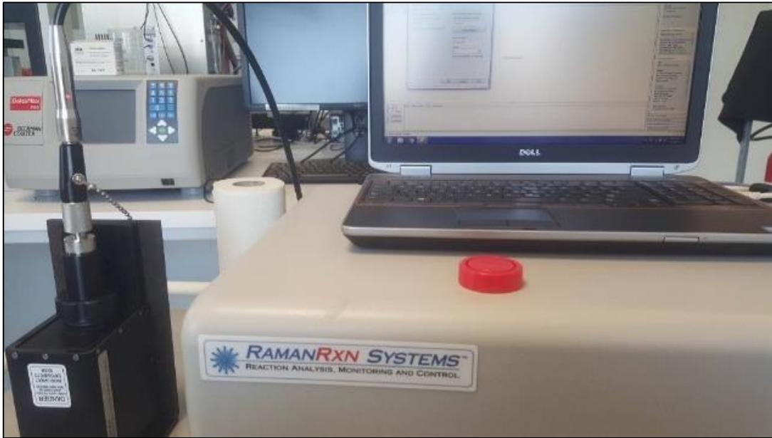
**Figure 29. Raman spectrometer used for analyzing cement samples**
