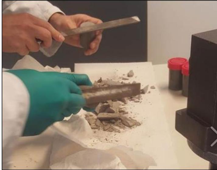
**Figure 77. Example of breakibroken samples and smoothing of the surfaces**
