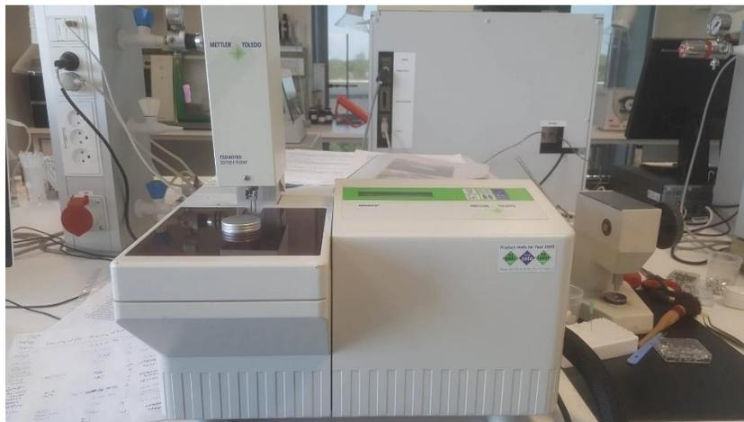
**Figure 57. DSC machine with autosampler used for the experiments**
