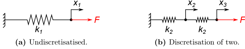
Figure 2.3: Modelling of the tensile stiffness with and without discretisation.
