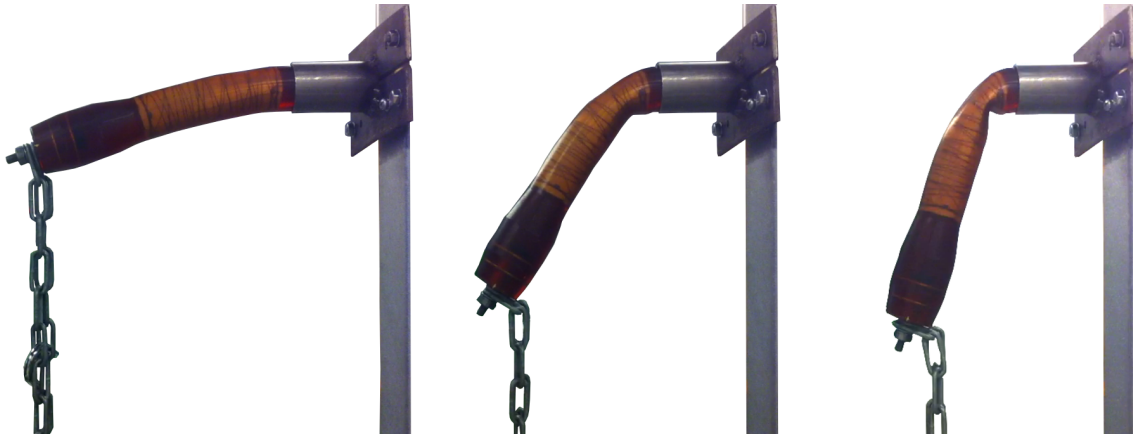
Figure I.3: The deflection at (from left) 5, 35 and 50 kg.
