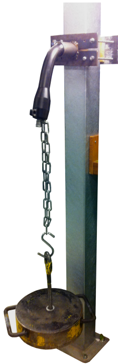
Figure 3.9: Setup for determining the bending stiffness
