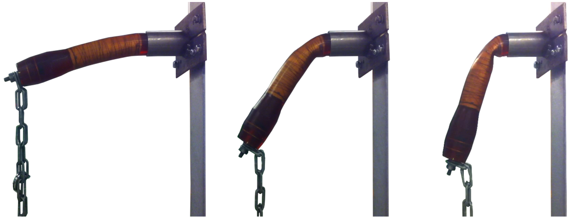
Figure 8.6: The deflection at (from left) 5, 35 and 50 kg. The collapse
