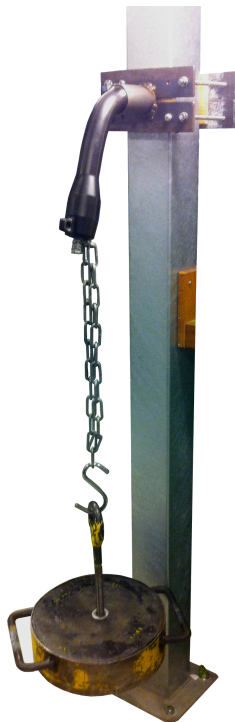
Figure E.1: Setup for determining the bending stiffness
