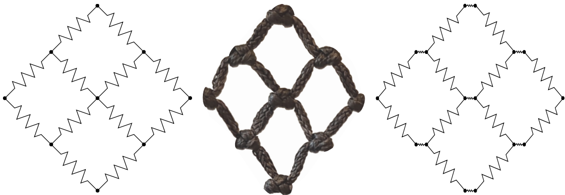
Figure 10.1: Left: current modelling of the net is showed. Middle: The net. Right: Suggested model.
