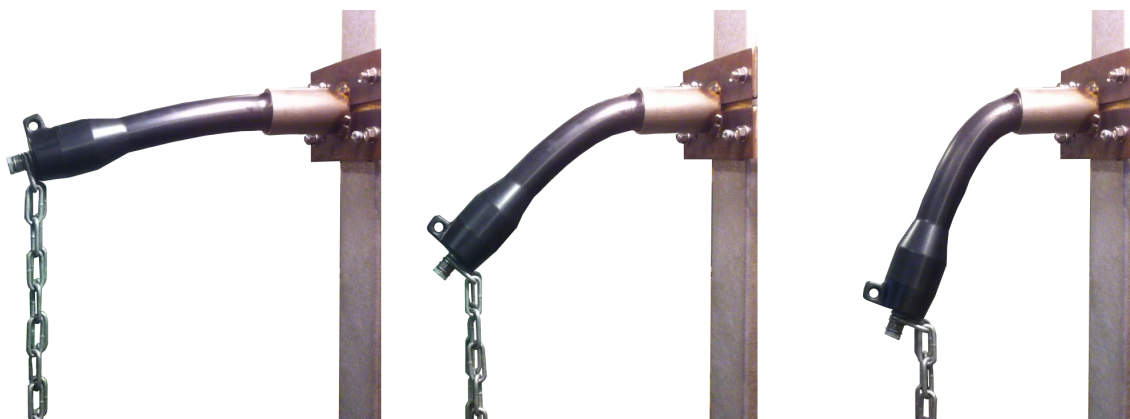
Figure E.5: The deflection at (from left) 5, 20 and 50 kg.
