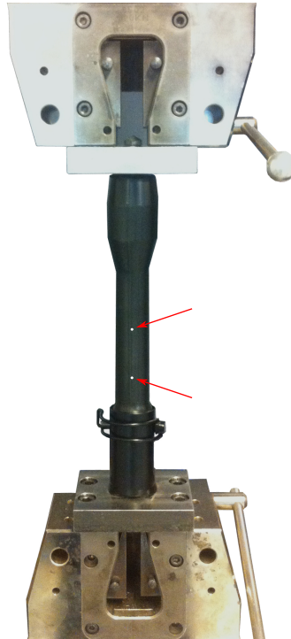
Figure D.1: The setup for the determination of the tensile stiffness of the rod.
