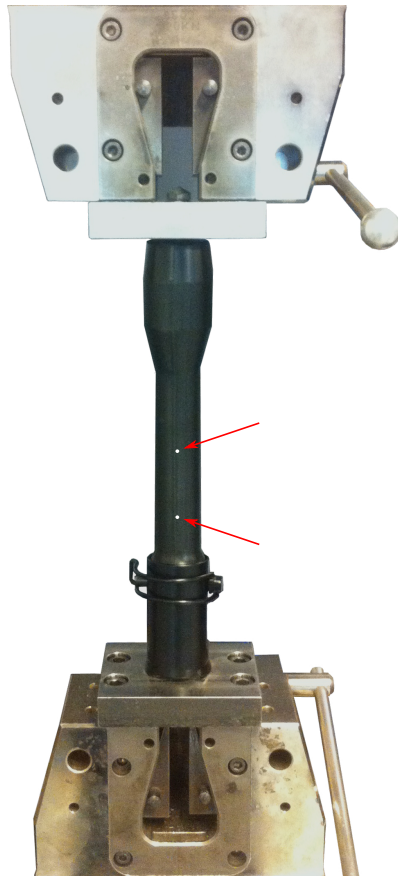
Figure 3.5: The setup for the determination of the tensile stiffness of the rod.
