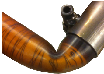
Figure 8.9: Collapse of the cross section.
